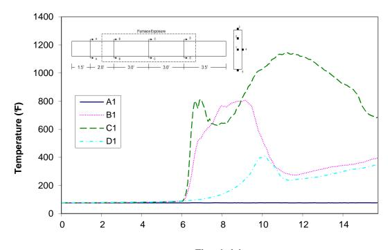
Time (min) Figure A-5: Temperature distribution in wood joist T1 at thermocouple location 1
