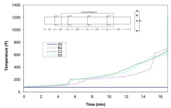
Figure A-48: Temperature distribution in wood joist T5 at thermocouple location 2
