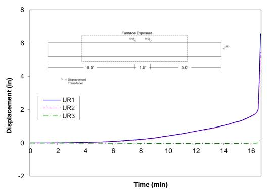
Figure A-31: Measured displacements recorded during fire resistance tests of wood joist T3
