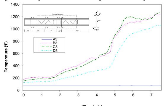
Time (min) Figure A-95: Temperature distribution in wood joist C1 at thermocouple location 3
