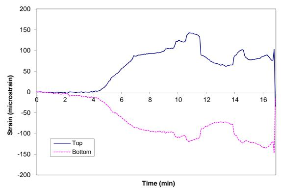
Figure A-52: Measured strains recorded during fire resistance tests of wood joist T5
