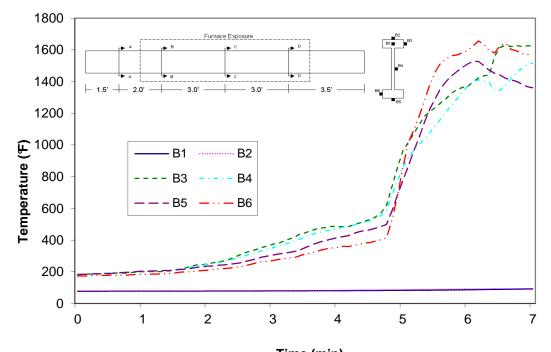
Time (min) Figure A-66: Temperature distribution in wood joist E2 at cross-section B
