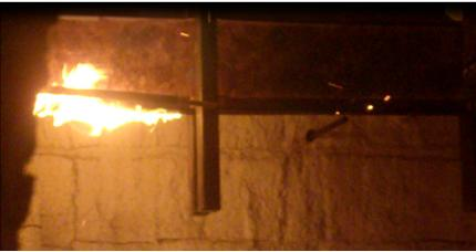
Figure B-16: Flame progression of joist E1 at time 04:14 (embers form on bottom cord at midspan)
