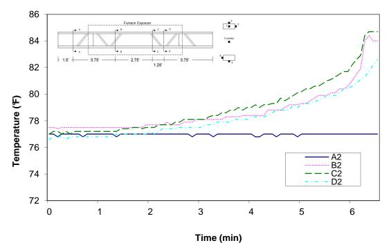
Figure A-117: Temperature distribution in wood joist H1 at thermocouple location 2
