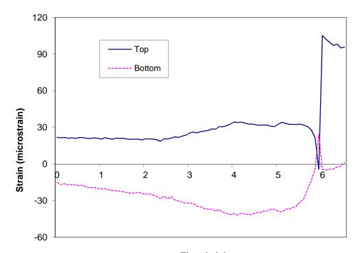
Time (min) Figure A-133: Measured strains recorded during fire resistance tests of wood joist H2
