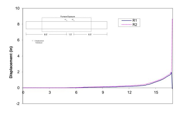
Time (min) Figure A-53: Measured displacements recorded during fire resistance tests of wood joist T5
