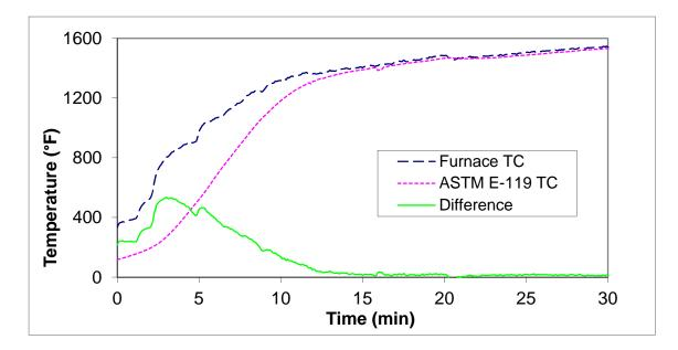
Figure 7: Comparison between the response of furnace and ASTM E-119 Thermocouples
