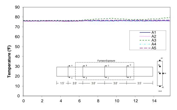
Time (min) Figure A-1: Temperature distribution in wood joist T1 at cross-section A
