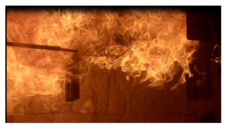
Figure B-20: Flame progression of joist E1 at time 04:48 (joist engulfed in flame)
