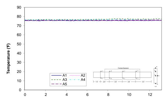
Time (min) Figure A-11: Temperature distribution in wood joist T2 at cross-section A
