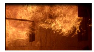
Image from video of flaming of web for I-joist fire test
