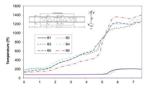
Time (min) Figure A-90: Temperature distribution in wood joist C1 at cross-section B
