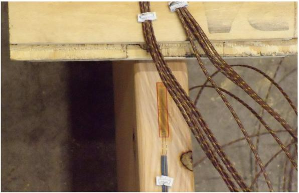
Figure B-3: Strain gauge mounted to top surface of joist T4
