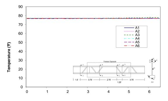
Time (min) Figure A-123: Temperature distribution in wood joist H2 at cross-section A
