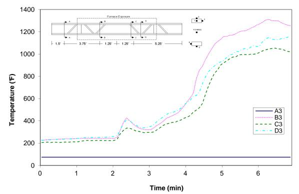
Figure A-153: Temperature distribution in wood joist H4 at thermocouple location 3
