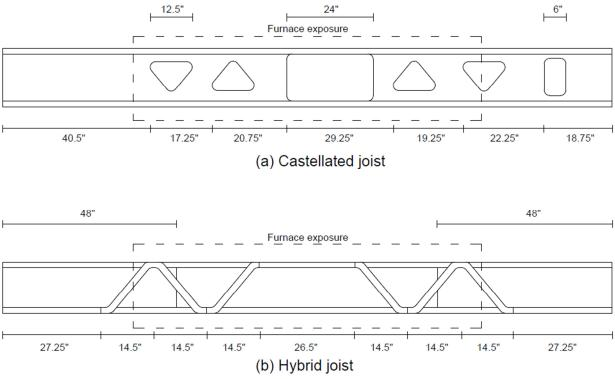
Figure 3: Engineered lumber cut-out orientation
