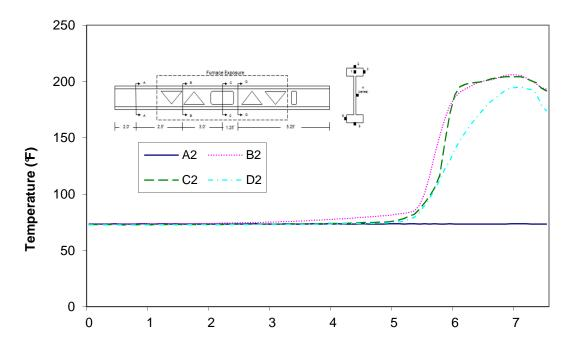
Time (min) Figure A-94: Temperature distribution in wood joist C1 at thermocouple location 2
