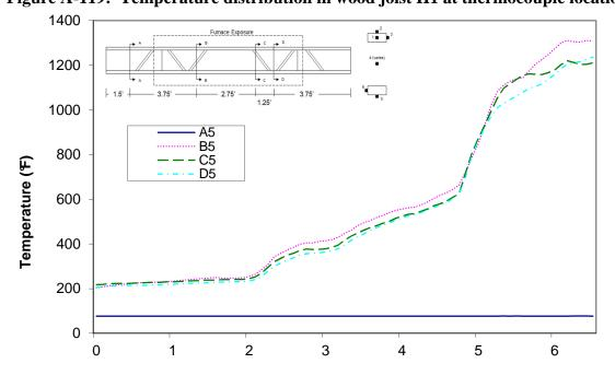
Time (min) Figure A-120: Temperature distribution in wood joist H1 at thermocouple location 5
