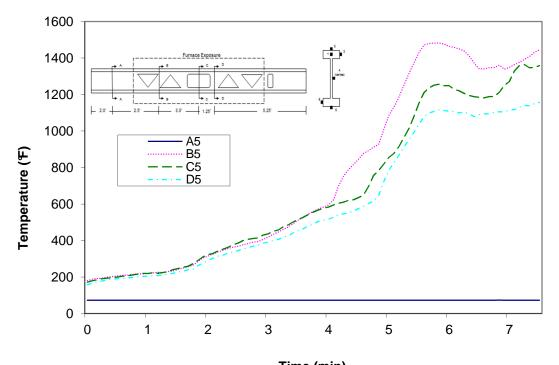
Time (min) Figure A-108: Temperature distribution in wood joist C2 at thermocouple location 5
