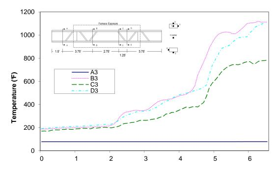
Time (min) Figure A-129: Temperature distribution in wood joist H2 at thermocouple location 3
