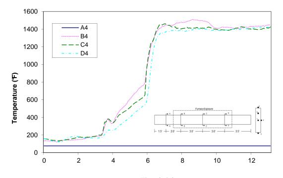
Time (min) Figure A-18: Temperature distribution in wood joist T2 at thermocouple location 4
