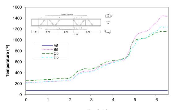
Time (min)Figure A-131: Temperature distribution in wood joist H2 at thermocouple location 5
