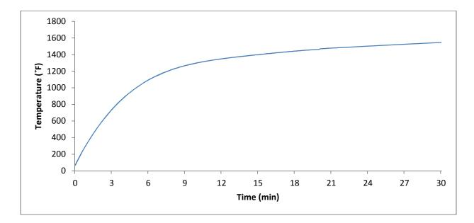
Figure 8: ASTM E-119 time-temperature curve used in fire tests
