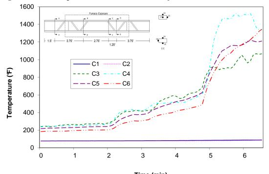
Time (min) Figure A-114: Temperature distribution in wood joist H1 at cross-section C
