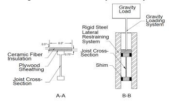
(c) Joist cross-sections with no lateral restraint (A-A) and with lateral restraint (B-B) Figure 2: Loading and restraining networks used in fire resistance tests
