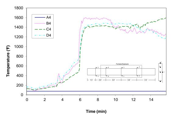
Figure A-8: Temperature distribution in wood joist T1 at thermocouple location 4
