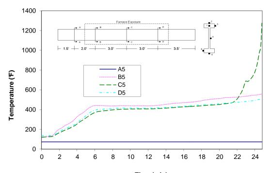
Time (min) Figure A-85: Temperature distribution in wood joist E3 at thermocouple location 5
