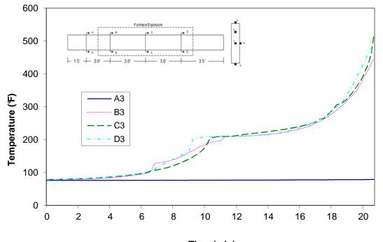
Time (min) Figure A-38: Temperature distribution in wood joist T4 at thermocouple location 3
