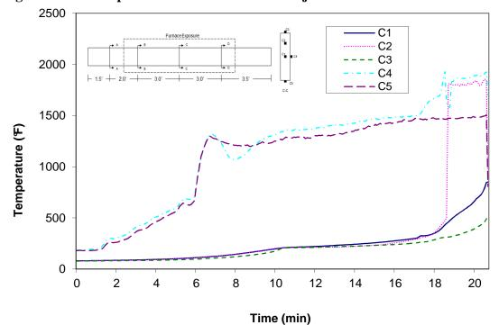
Figure A-34: Temperature distribution in wood joist T4 at cross-section C
