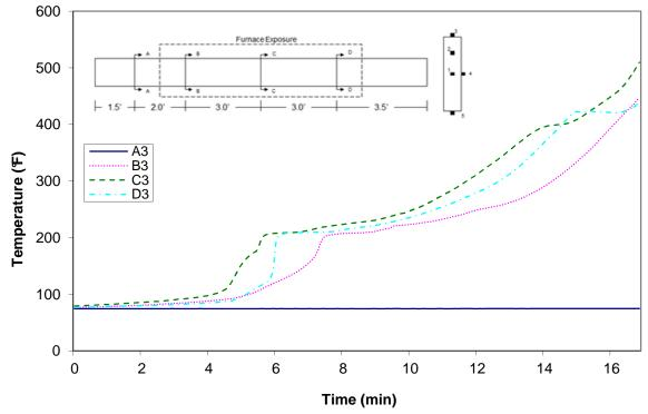
Figure A-49: Temperature distribution in wood joist T5 at thermocouple location 3
