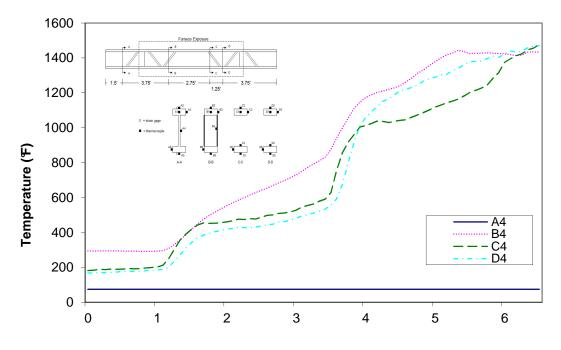
Time (min) Figure A-142: Temperature distribution in wood joist H3 at thermocouple location 4
