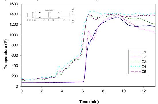
Figure A-13: Temperature distribution in wood joist T2 at cross-section C
