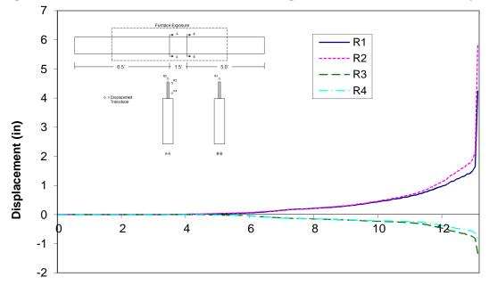
Time (min) Figure A-21: Measured displacements recorded during fire resistance tests of wood joist T2
