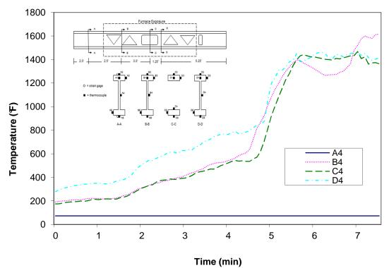
Figure A-107: Temperature distribution in wood joist C2 at thermocouple location 4
