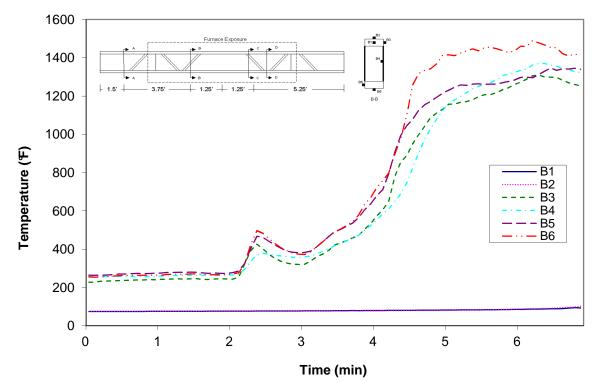
Figure A-147: Temperature distribution in wood joist H4 at cross-section A
