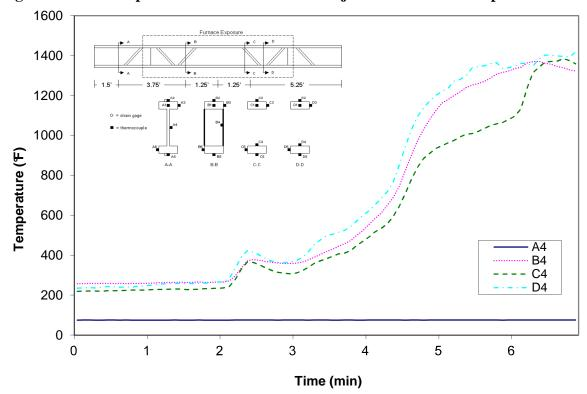
Figure A-154: Temperature distribution in wood joist H4 at thermocouple location 4
