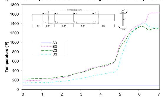
Time (min) Figure A-71: Temperature distribution in wood joist E2 at thermocouple location 3
