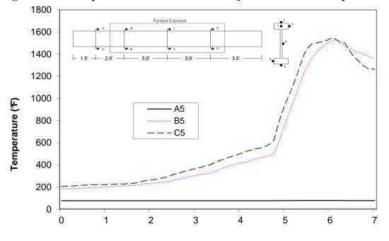
Time (min) Figure A-73: Temperature distribution in wood joist E2 at thermocouple location 5
