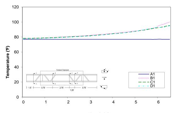
Time (min) Figure A-127: Temperature distribution in wood joist H2 at thermocouple location 1
