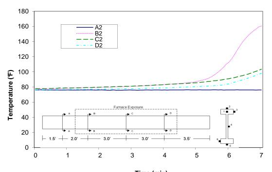
Time (min) Figure A-59: Temperature distribution in wood joist E1 at thermocouple location 2
