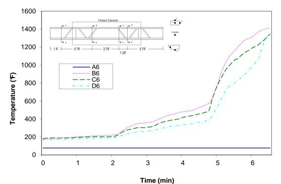
Figure A-121: Temperature distribution in wood joist H1 at thermocouple location 6
