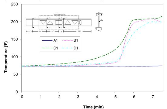
Figure A-93: Temperature distribution in wood joist C1 at thermocouple location 1
