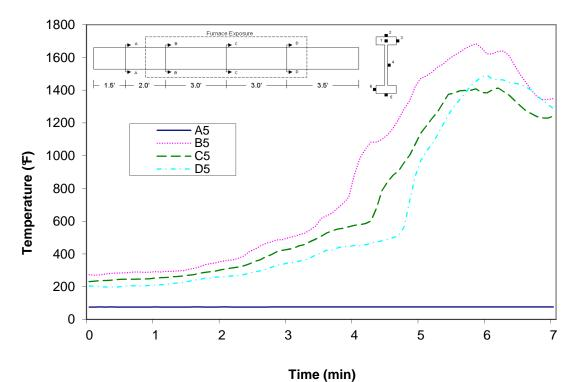
Figure A-62: Temperature distribution in wood joist E1 at thermocouple location 5
