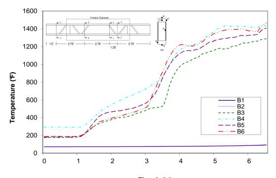
Time (min) Figure A-136: Temperature distribution in wood joist H3 at cross-section B
