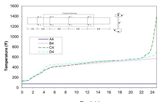
Time (min) Figure A-84: Temperature distribution in wood joist E3 at thermocouple location 4
