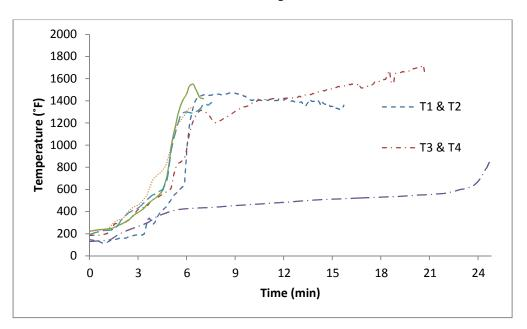
Figure 12: Comparison of averaged temperatures in different joist types at thermocouple location 4
