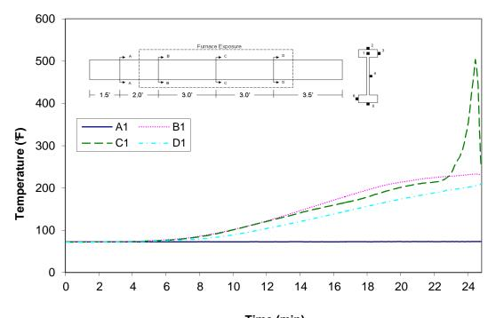
Time (min) Figure A-81: Temperature distribution in wood joist E3 at thermocouple location 1
