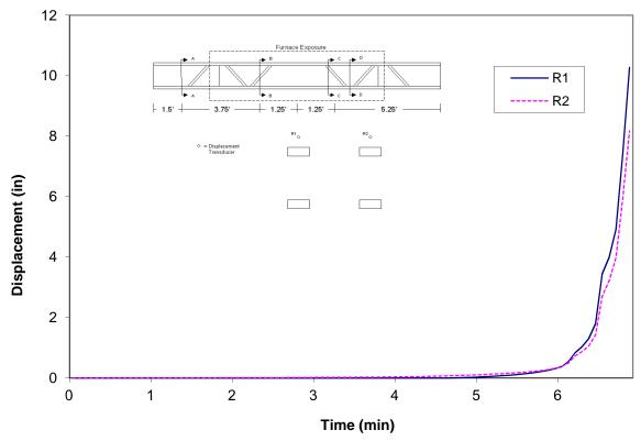
Figure A-158: Measured displacements recorded during fire resistance tests of wood
