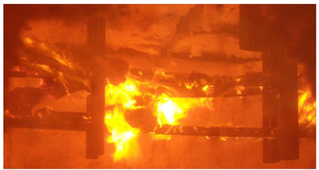
Figure B-9: Castellated joist (C2) after failure
