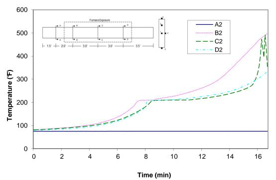
Figure A-27: Temperature distribution in wood joist T3 at thermocouple location 2
