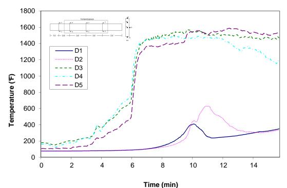
Figure A-4: Temperature distribution in wood joist T1 at cross-section D
