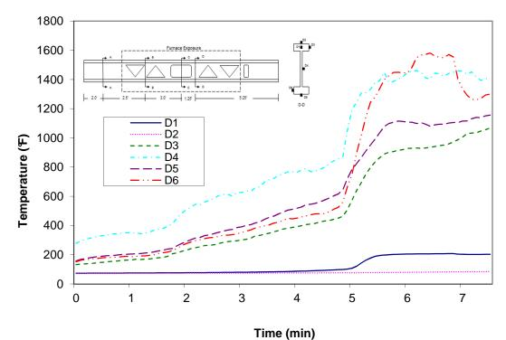
Figure A-103: Temperature distribution in wood joist C2 at cross-section D
