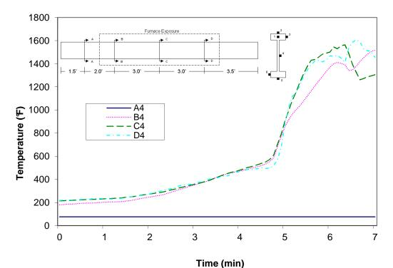
Figure A-72: Temperature distribution in wood joist E2 at thermocouple location 4
