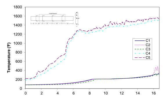
Time (min) Figure A-24: Temperature distribution in wood joist T3 at cross-section C
