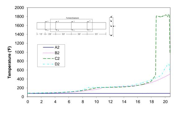
Time (min) Figure A-37: Temperature distribution in wood joist T4 at thermocouple location 2
