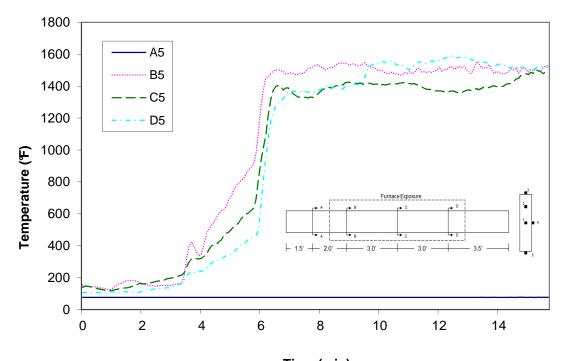
Time (min) Figure A-9: Temperature distribution in wood joist T1 at thermocouple location 5
