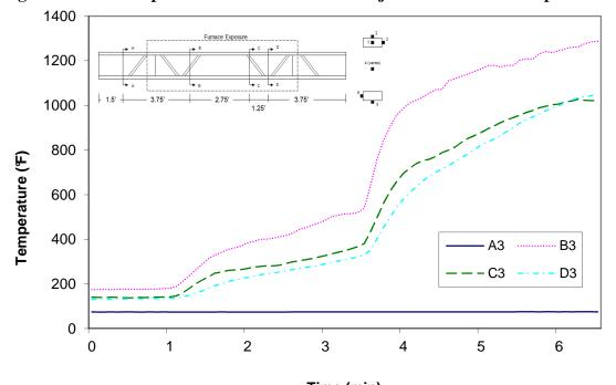
Time (min) Figure A-141: Temperature distribution in wood joist H3 at thermocouple location 3
