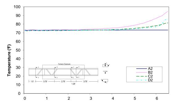
Time (min) Figure A-140: Temperature distribution in wood joist H3 at thermocouple location 2
