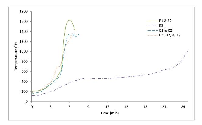
Figure 14: Comparison of averaged temperatures in different joist types at thermocouple location 6
