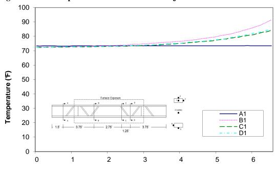
Time (min) Figure A-139: Temperature distribution in wood joist H3 at thermocouple location 1
