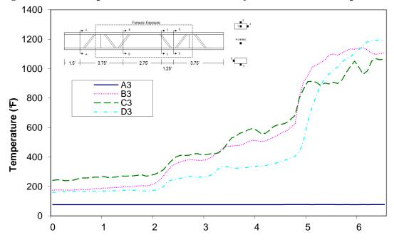
Time (min) Figure A-118: Temperature distribution in wood joist H1 at thermocouple location 3
