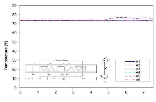
Time (min) Figure A-89: Temperature distribution in wood joist C1 at cross-section A
