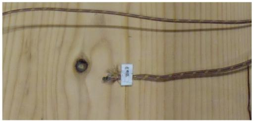
**Figure B-2:** Thermocouple mounted to side of traditional joist T2
