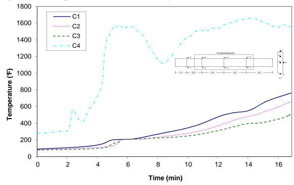
Figure A-45: Temperature distribution in wood joist T5 at cross-section C
