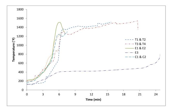
Figure 13: Comparison of averaged temperatures in different joist types at thermocouple location 5
