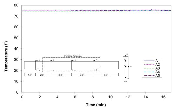
Figure A-43: Temperature distribution in wood joist T5 at cross-section A
