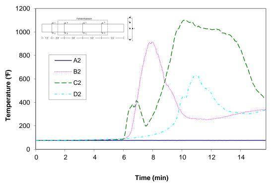
Figure A-6: Temperature distribution in wood joist T1 at thermocouple location 2
