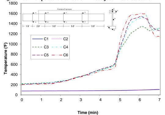
Figure A-67: Temperature distribution in wood joist E2 at cross-section C
