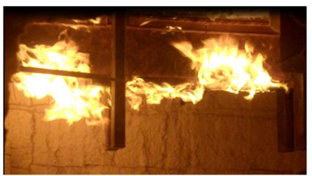
Figure B-19: Flame progression of joist E1 at time 04:33 (flame appears at the location of embers)
