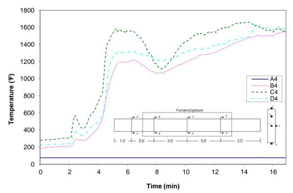
Figure A-50: Temperature distribution in wood joist T5 at thermocouple location 4
