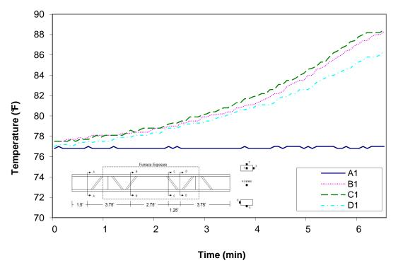
Figure A-116: Temperature distribution in wood joist H1 at thermocouple location 1
