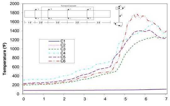
Figure A-55: Temperature distribution in wood joist E1 at cross-section B
