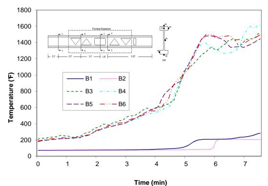
Figure A-101: Temperature distribution in wood joist C2 at cross-section B
