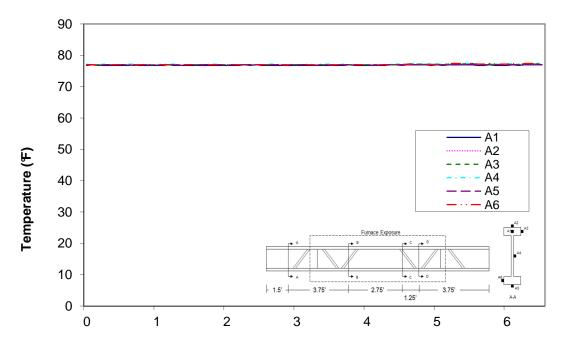
Time (min) Figure A-112: Temperature distribution in wood joist H1 at cross-section A
