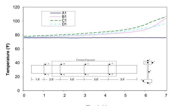
Time (min) Figure A-58: Temperature distribution in wood joist E1 at thermocouple location 1
