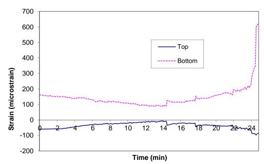
Figure A-87: Measured strains recorded during fire resistance tests of wood joist E3
