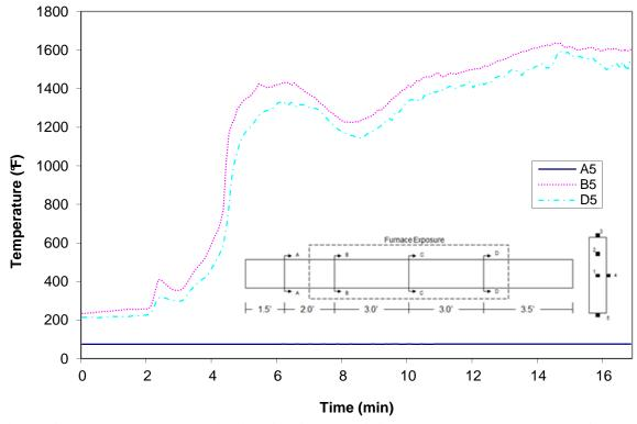
Figure A-51: Temperature distribution in wood joist T5 at thermocouple location 5
