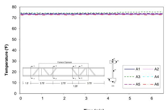
Time (min) Figure A-135: Temperature distribution in wood joist H3 at cross-section A
