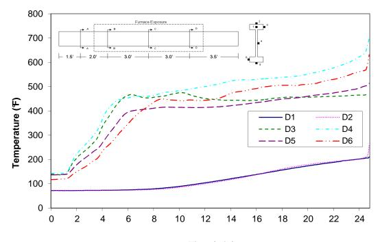
Time (min) Figure A-80: Temperature distribution in wood joist E3 at cross-section D
