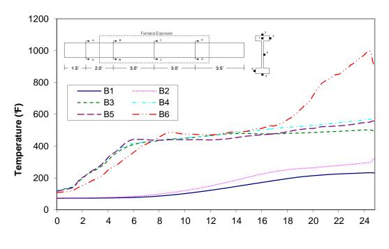
Time (min) Figure A-78: Temperature distribution in wood joist E3 at cross-section B
