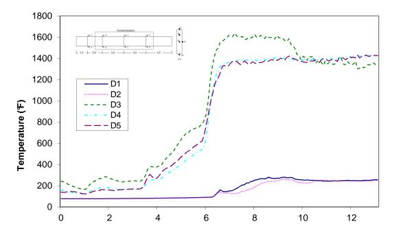
Time (min) Figure A-14: Temperature distribution in wood joist T2 at cross-section D
