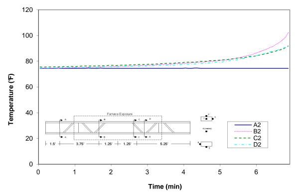
Figure A-151: Temperature distribution in wood joist H4 at thermocouple location 1
