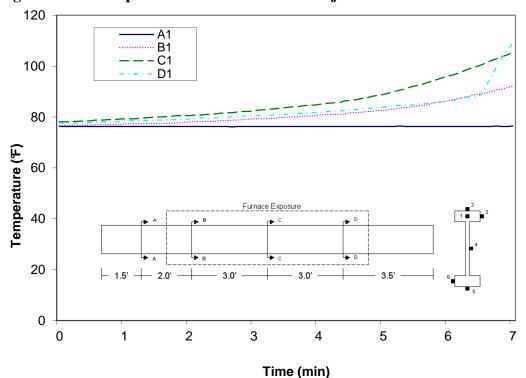
Figure A-69: Temperature distribution in wood joist E2 at thermocouple location 1
