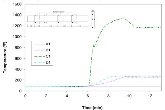
Figure A-15: Temperature distribution in wood joist T2 at thermocouple location 1
