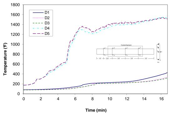
Figure A-25: Temperature distribution in wood joist T3 at cross-section D
