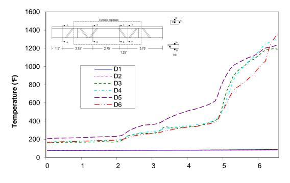
Time (min) Figure A-115: Temperature distribution in wood joist H1 at cross-section D
