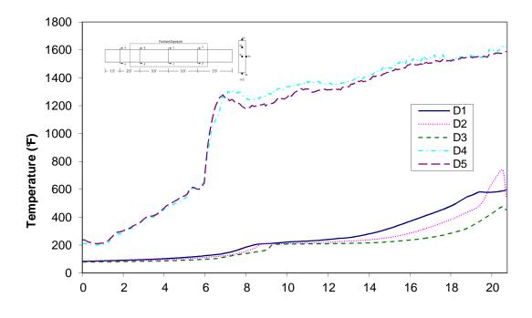
Time (min) Figure A-35: Temperature distribution in wood joist T4 at cross-section D
