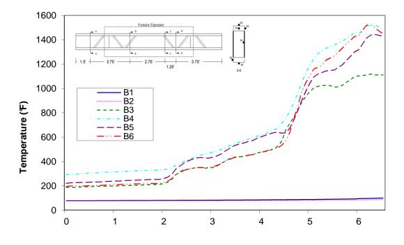
Time (min) Figure A-124: Temperature distribution in wood joist H2 at cross-section B
