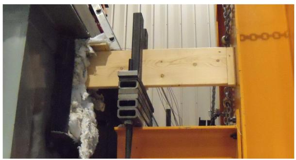
Figure B-4: Joist T4 axially restrained against test frame and laterally restrained at support
