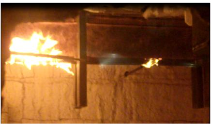
Figure B-17: Flame progression of joist E1 at time 04:16 (flame appears at the location of embers)
