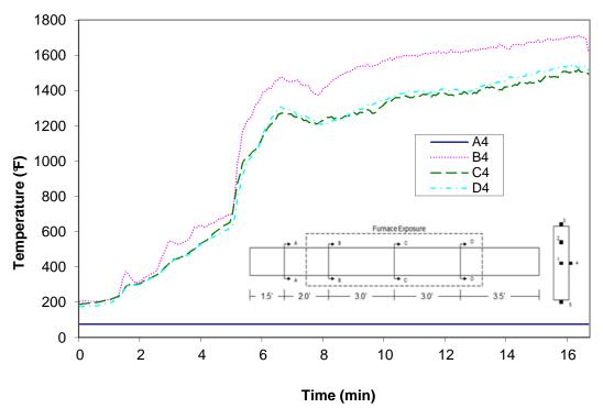
Figure A-29: Temperature distribution in wood joist T3 at thermocouple location 4
