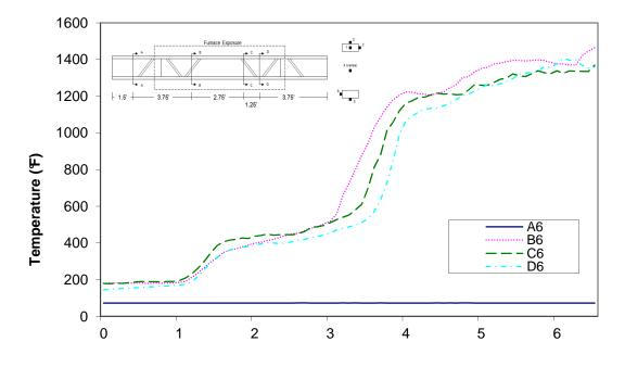
Time (min) Figure A-144: Temperature distribution in wood joist H3 at thermocouple location 6
