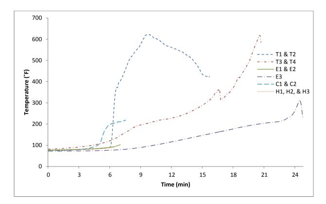
Figure 9: Comparison of averaged temperatures in different joist types at thermocouple location 1
