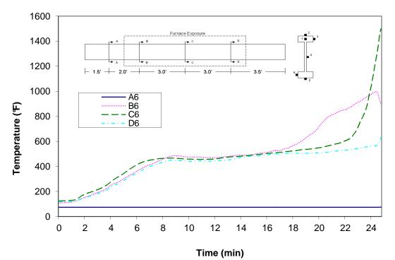
Figure A-86: Temperature distribution in wood joist E3 at thermocouple location 6
