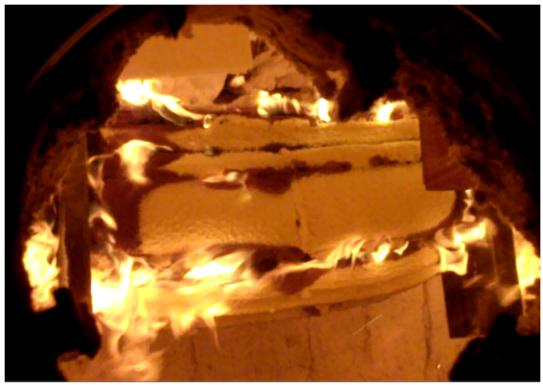
Figure B-12: Joist E3 immediately after failure
