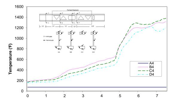
Time (min) Figure A-96: Temperature distribution in wood joist C1 at thermocouple location 4
