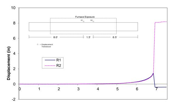
Time (min) Figure A-111: Measured displacements recorded during fire resistance tests of wood joist C2
