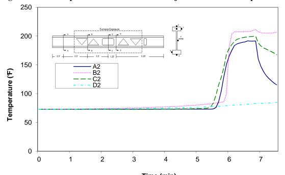
Time (min) Figure A-105: Temperature distribution in wood joist C2 at thermocouple location 2
