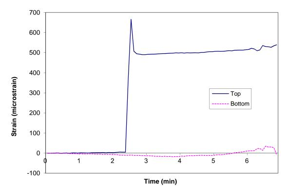
Figure A-157: Measured strains recorded during fire resistance tests of wood joist H4
