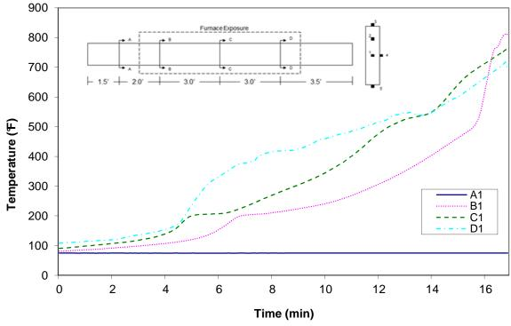
Figure A-47: Temperature distribution in wood joist T5 at thermocouple location 1
