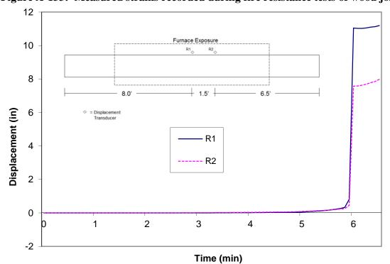
Figure A-134: Measured displacements recorded during fire resistance tests of wood joist H2
