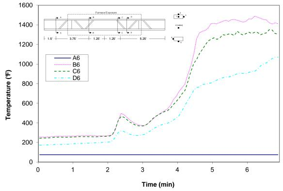
Figure A-156: Temperature distribution in wood joist H4 at thermocouple location 6
