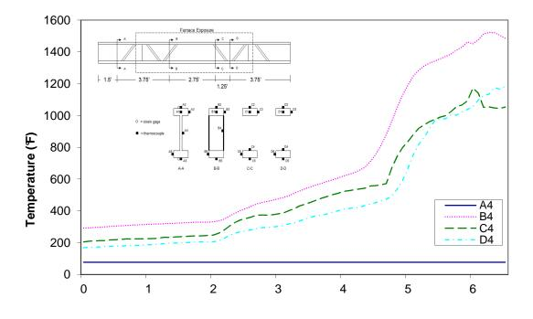
Time (min) Figure A-130: Temperature distribution in wood joist H2 at thermocouple location 4
