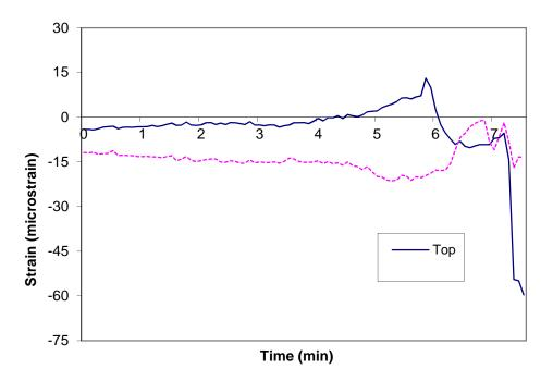
Figure 15: Measured representative strains during fire resistance test of joist C2
