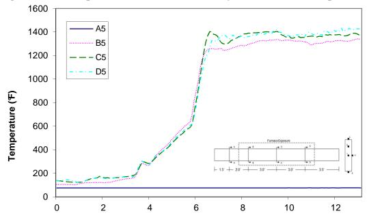
Time (min) Figure A-19: Temperature distribution in wood joist T2 at thermocouple location 5
