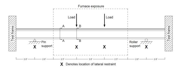
(b) Loading and restraining network used for axially restrained joists
