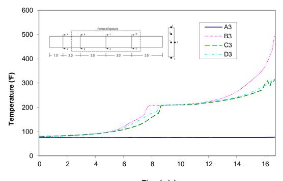
Time (min) Figure A-28: Temperature distribution in wood joist T3 at thermocouple location 3
