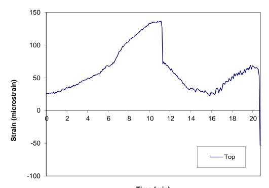
Time (min) Figure A-41: Measured strains recorded during fire resistance tests of wood joist T4
