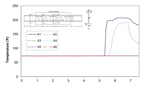
Time (min) Figure A-100: Temperature distribution in wood joist C2 at cross-section A
