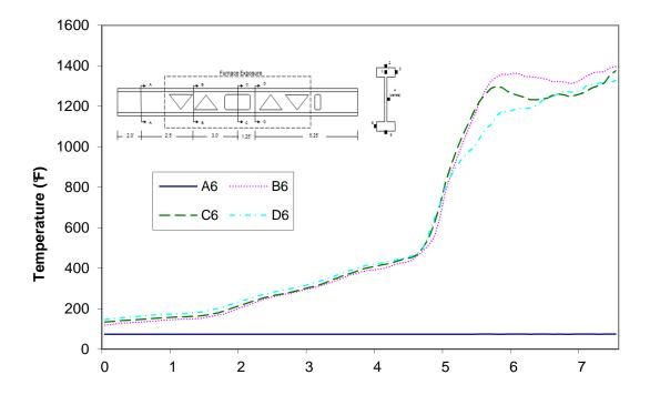
Time (min) Figure A-98: Temperature distribution in wood joist C1 at thermocouple location 6
