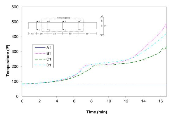
Figure A-26: Temperature distribution in wood joist T3 at thermocouple location 1
