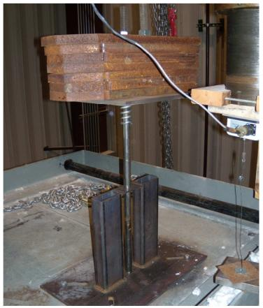
Figure B-6: Loading and lateral restraining system for joist E1
