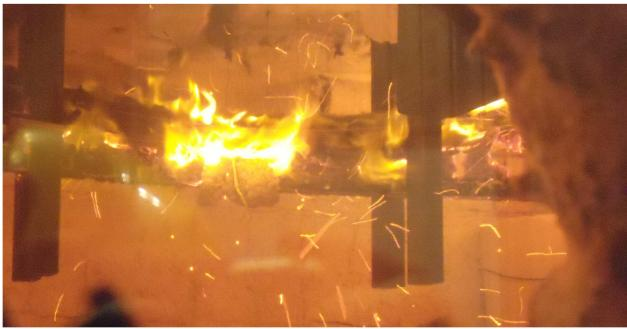
Figure B-8: Engineered joist (E1) after failure
