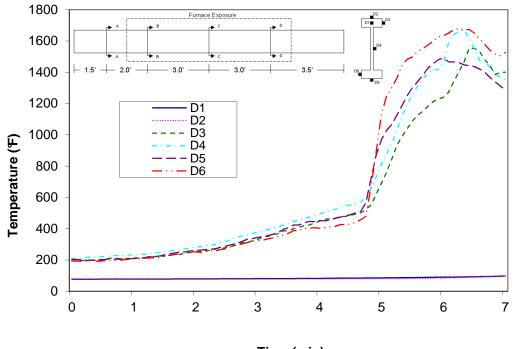
Time (min) Figure A-57: Temperature distribution in wood joist E1 at cross-section D
