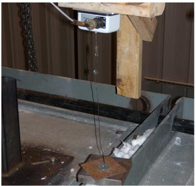
Figure B-5: Vertical displacement transducer connected to joist at midspan
