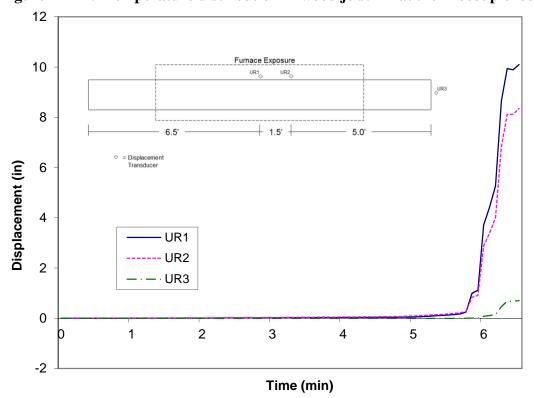
Figure A-122: Measured displacements recorded during fire resistance tests of wood joist H1
