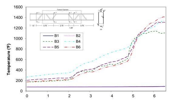
Time (min) Figure A-113: Temperature distribution in wood joist H1 at cross-section B
