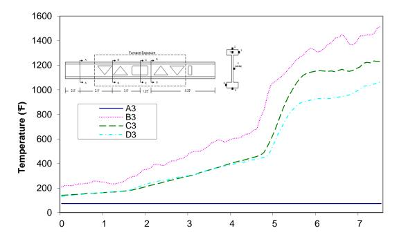
Time (min) Figure A-106: Temperature distribution in wood joist C2 at thermocouple location 3
