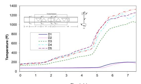
Time (min) Figure A-92: Temperature distribution in wood joist C1 at cross-section D
