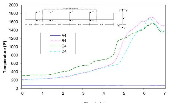
Time (min) Figure A-61: Temperature distribution in wood joist E1 at thermocouple location 4
