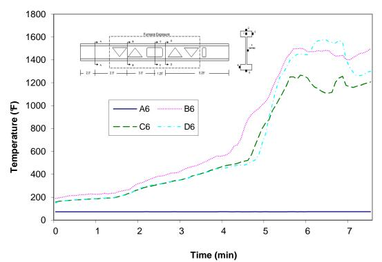
Figure A-109: Temperature distribution in wood joist C2 at thermocouple location 6
