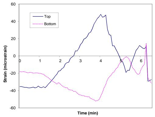
Figure A-145: Measured strains recorded during fire resistance tests of wood joist H3
