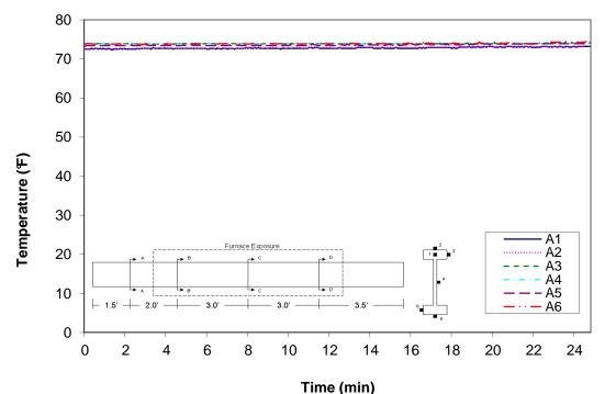
Figure A-77: Temperature distribution in wood joist E3 at cross-section A
