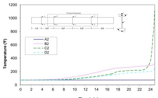
Time (min) Figure A-82: Temperature distribution in wood joist E3 at thermocouple location 2
