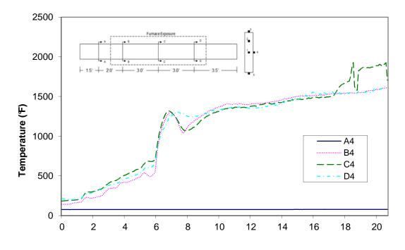
Time (min) Figure A-39: Temperature distribution in wood joist T4 at thermocouple location 4
