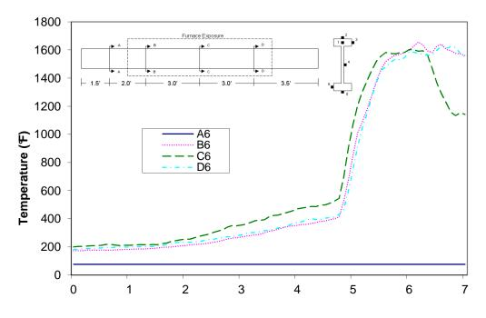
Time (min) Figure A-74: Temperature distribution in wood joist E2 at thermocouple location 6
