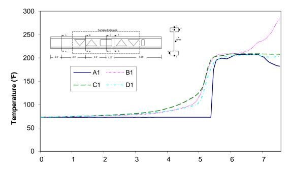
Time (min) Figure A-104: Temperature distribution in wood joist C2 at thermocouple location 1
