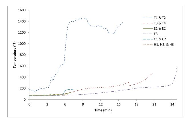
Figure 10: Comparison of averaged temperatures in different joist types at thermocouple location 2
