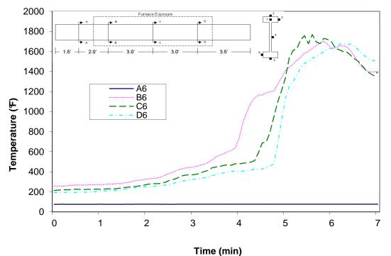
Figure A-63: Temperature distribution in wood joist E1 at thermocouple location 6
