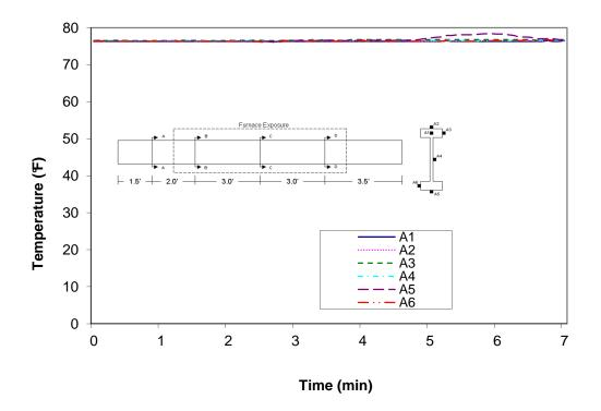
Figure A-65: Temperature distribution in wood joist E2 at cross-section A
