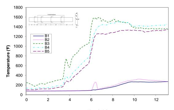
Time (min) Figure A-12: Temperature distribution in wood joist T2 at cross-section B
