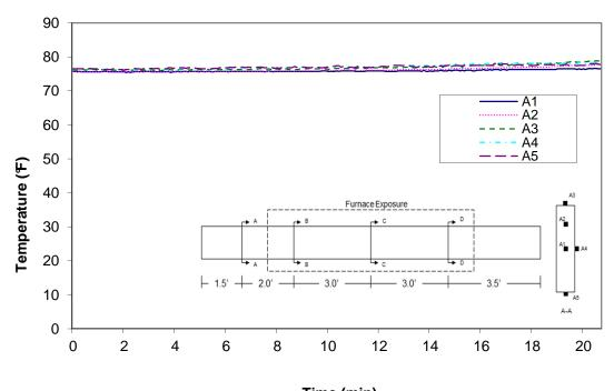
Time (min) Figure A-32: Temperature distribution in wood joist T4 at cross-section A
