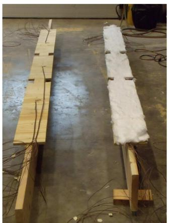
Figure B-1: Joists T3 (right) and T4 (left) with sheathing attached
