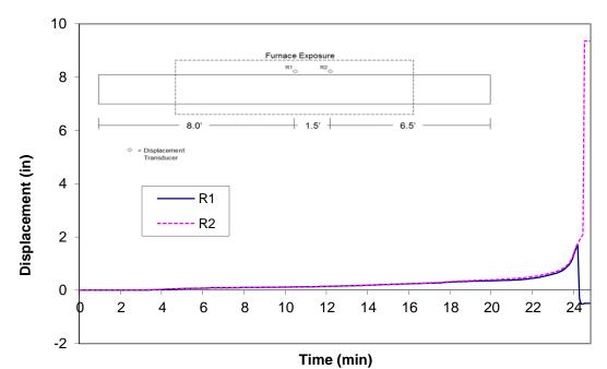
Figure A-88: Measured displacements recorded during fire resistance tests of wood joist E3
