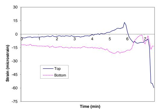
Figure A-110: Measured strains recorded during fire resistance tests of wood joist C2
