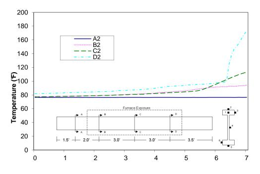
Time (min) Figure A-70: Temperature distribution in wood joist E2 at thermocouple location 2
