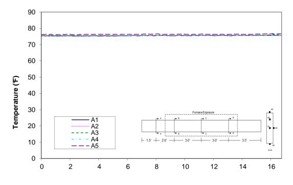
Time (min) Figure A-22: Temperature distribution in wood joist T3 at cross-section A
