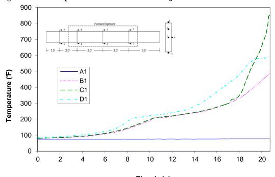
Time (min) Figure A-36: Temperature distribution in wood joist T4 at thermocouple location 1
