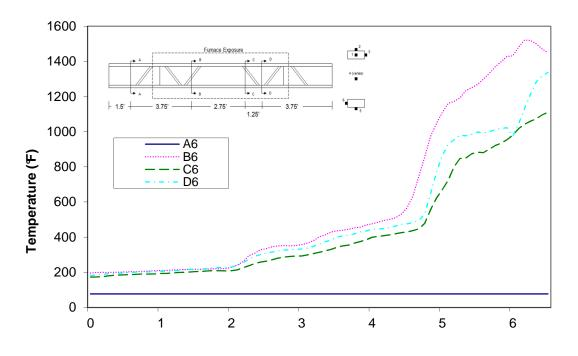
Time (min) Figure A-132: Temperature distribution in wood joist H2 at thermocouple location 6
