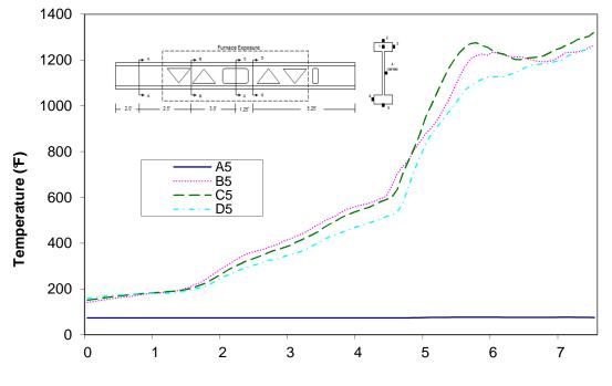
Time (min) Figure A-97: Temperature distribution in wood joist C1 at thermocouple location 5
