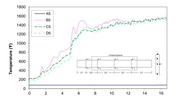
Time (min) Figure A-30: Temperature distribution in wood joist T3 at thermocouple location 5
