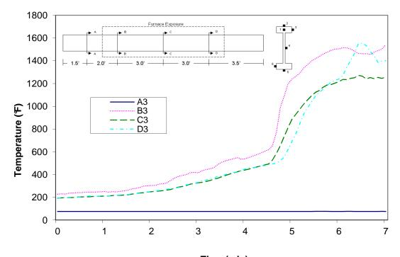
Time (min) Figure A-60: Temperature distribution in wood joist E1 at thermocouple location 3
