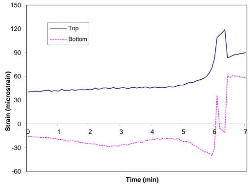
Figure A-75: Measured strains recorded during fire resistance tests of wood joist E2
