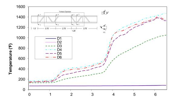
Time (min) Figure A-138: Temperature distribution in wood joist H3 at cross-section D
