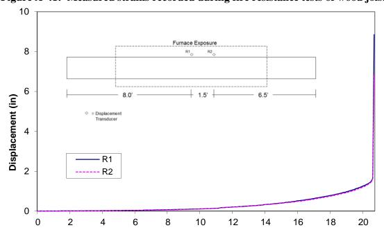
Time (min) Figure A-42: Measured displacements recorded during fire resistance tests of wood joist T4
