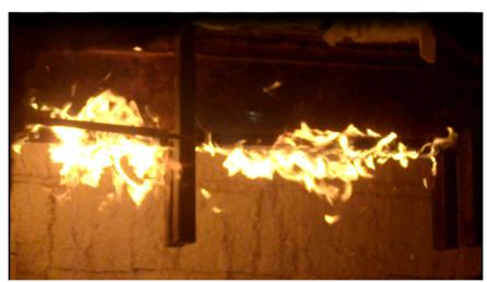
Figure B-18: Flame progression of joist E1 at time 04:29 (embers form on top cord)
