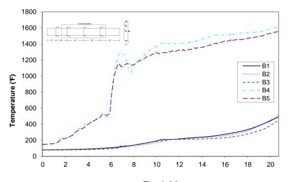
Time (min) Figure A-33: Temperature distribution in wood joist T4 at cross-section B
