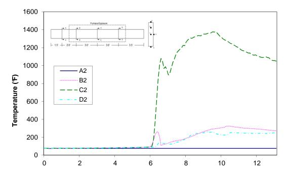
Time (min) Figure A-16: Temperature distribution in wood joist T2 at thermocouple location 2
