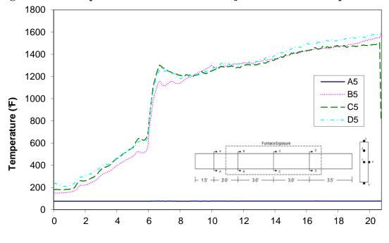
Time (min) Figure A-40: Temperature distribution in wood joist T4 at thermocouple location 5
