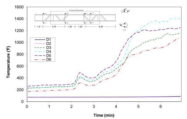
Figure A-149: Temperature distribution in wood joist H4 at cross-section C
