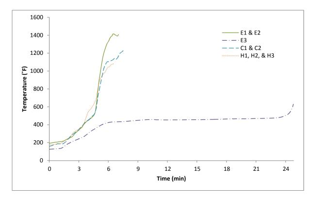
Figure 11: Comparison of averaged temperatures in different joist types at thermocouple location 3
