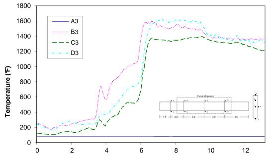
Time (min) Figure A-17: Temperature distribution in wood joist T2 at thermocouple location 3
