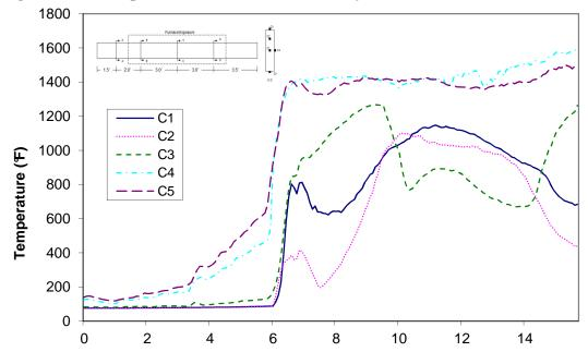
Figure A-2: Temperature distribution in wood joist T1 at cross-section B
