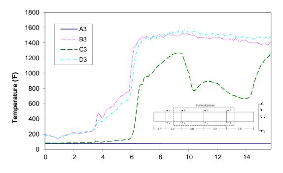
Time (min) Figure A-7: Temperature distribution in wood joist T1 at thermocouple location 3
