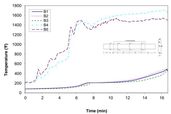
Figure A-23: Temperature distribution in wood joist T3 at cross-section B
