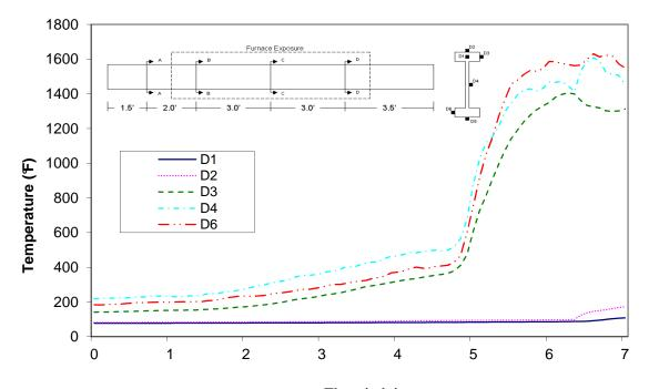
Time (min) Figure A-68: Temperature distribution in wood joist E2 at cross-section D
