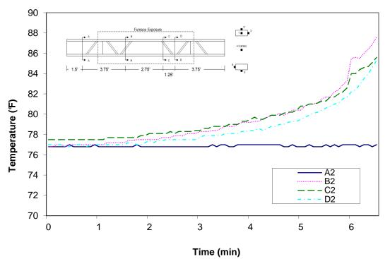
Figure A-128: Temperature distribution in wood joist H2 at thermocouple location 2
