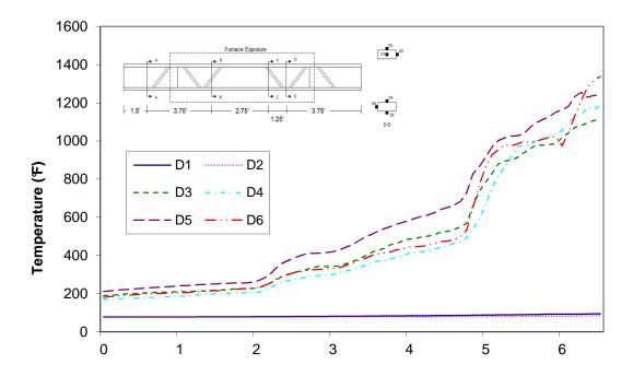
Time (min) Figure A-126: Temperature distribution in wood joist H2 at cross-section D
