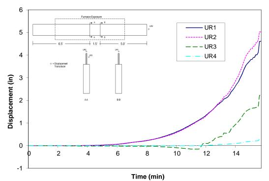
Figure A-10: Measured displacements recorded during fire resistance tests of wood joist T1
