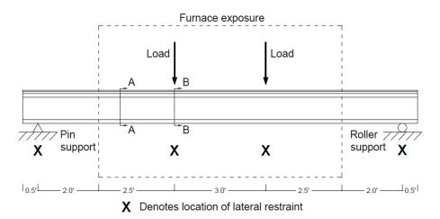
(a) Loading and restraining network used for axially unrestrained joists
