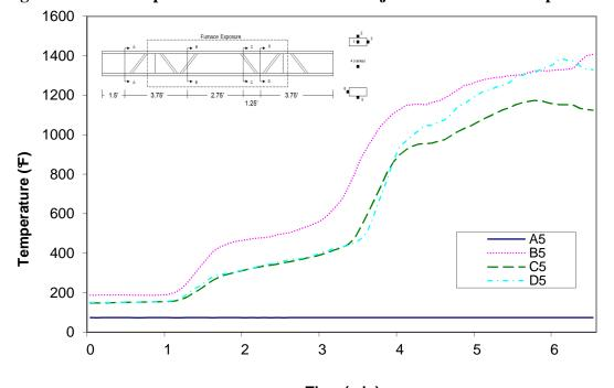
Time (min) Figure A-143: Temperature distribution in wood joist H3 at thermocouple location 5
