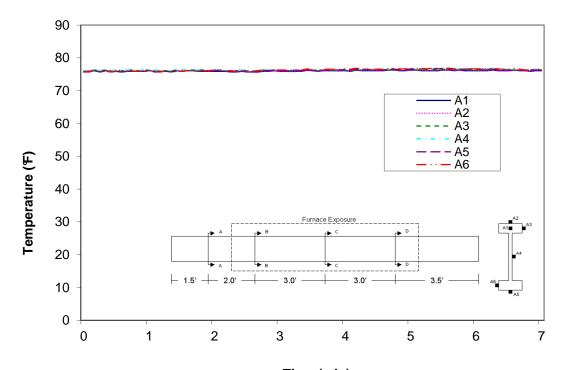
Time (min) Figure A-54: Temperature distribution in wood joist E1 at cross-section A
