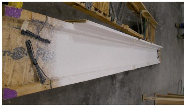
Figure B-11: Joist E3 with intumescent coating
