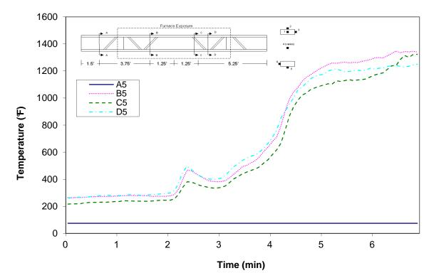
Figure A-155: Temperature distribution in wood joist H4 at thermocouple location 5
