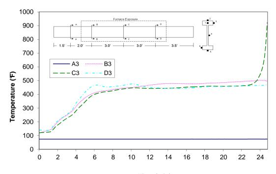
Time (min) Figure A-83: Temperature distribution in wood joist E3 at thermocouple location 3
