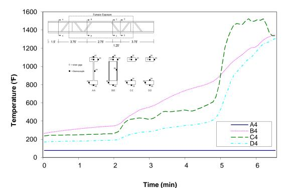
Figure A-119: Temperature distribution in wood joist H1 at thermocouple location 4
