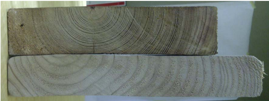
Figure 99. Comparison of the modern 2 x10 to the old 2 x 8.
