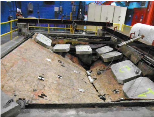
Figure 45. Unexposed side after collapse
