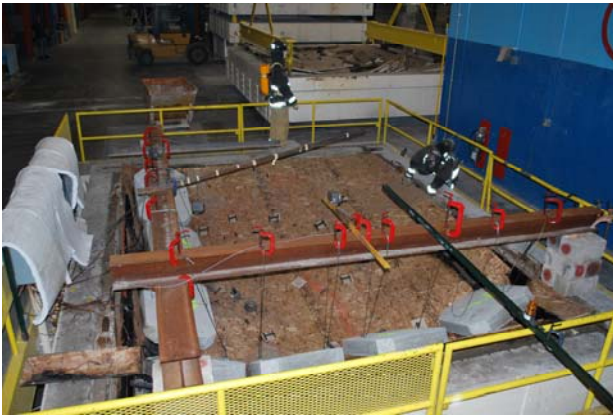
Figure 33. Unexposed side after collapse
