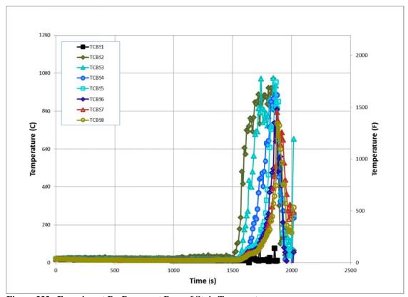
**Figure 333.** Experiment B - Basement Base of Stair Temperatures
