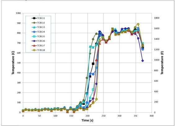
Figure 104. Experiment 3 - Basement Center Temperatures
