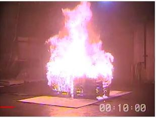
Figure 26. Conditions at 10:00 (600 s) – 3600 kW
