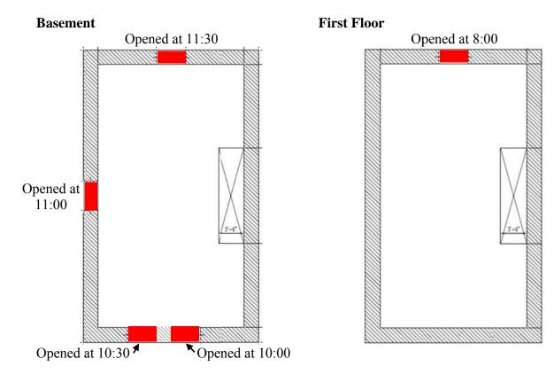
Figure 50. Sequenced Ventilation Details
