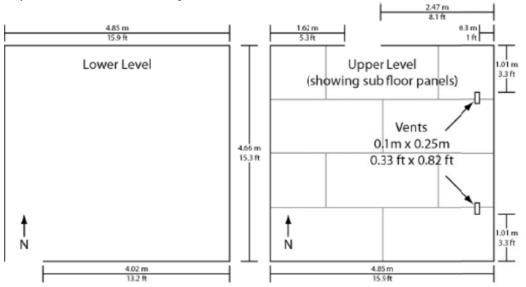
Figure 11. Floor plan of the upper and lower levels of the structures.
