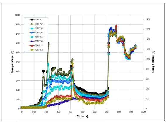
Figure 131. Experiment 4 - First Floor Top of Stair Temperatures
