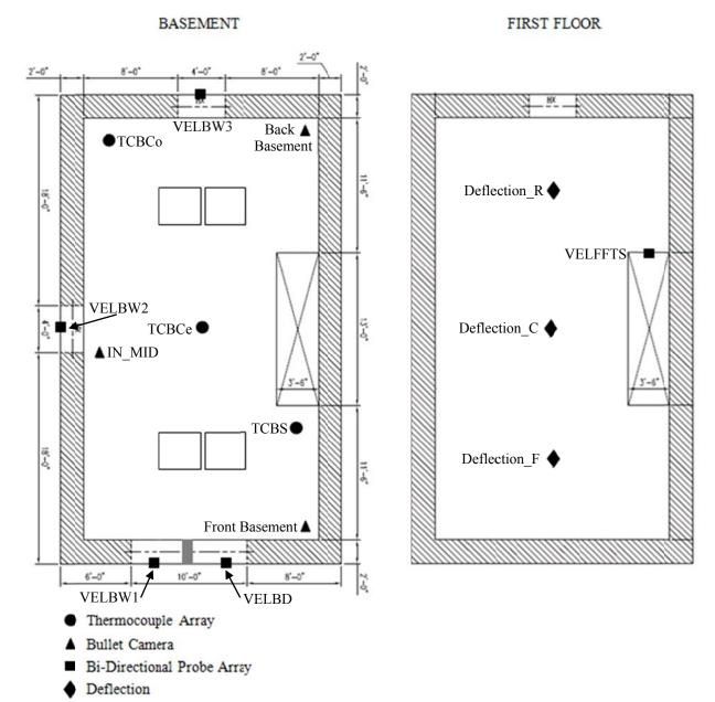
Figure 293. Measurement Locations and Labels
