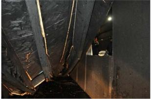
Figure 325 Mechanical separations of the web to flange connections, and flange member rupture.
