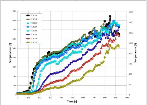
Figure 377. Experiment D - Basement Corner Temperatures
