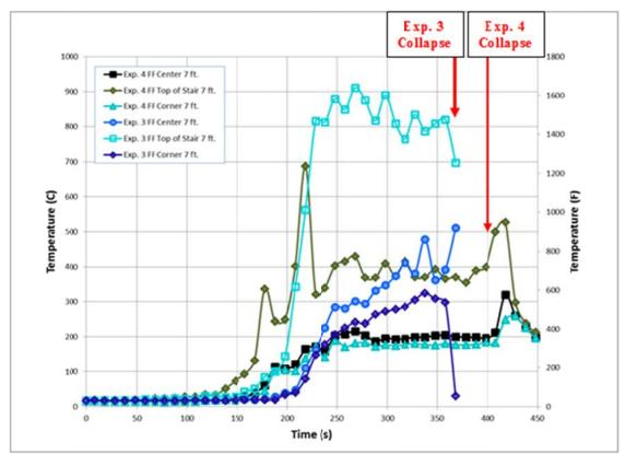
Figure 399. Experiment 3 and 4 Comparison of First Floor Temperatures at 7 ft. above the floor
