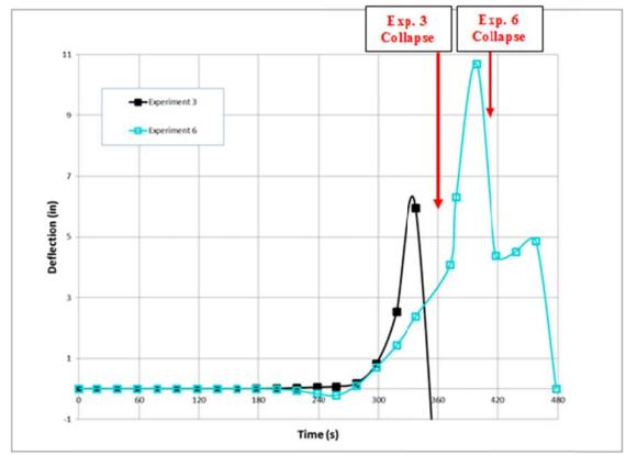
Figure 410 shows the deflection during Experiments 3 and 6. Both Experiments have approximately the same time to onset of deflection. Due to the smaller load Experiment 6 had a slightly slower rate of deflection leading up to collapse which accounts for the 49 seconds difference in collapse times. Ultimately the load on the floor system did not play a significant role in determining the time to collapse but rather the degradation of the floor system as it was consumed and weakened by the fire.
