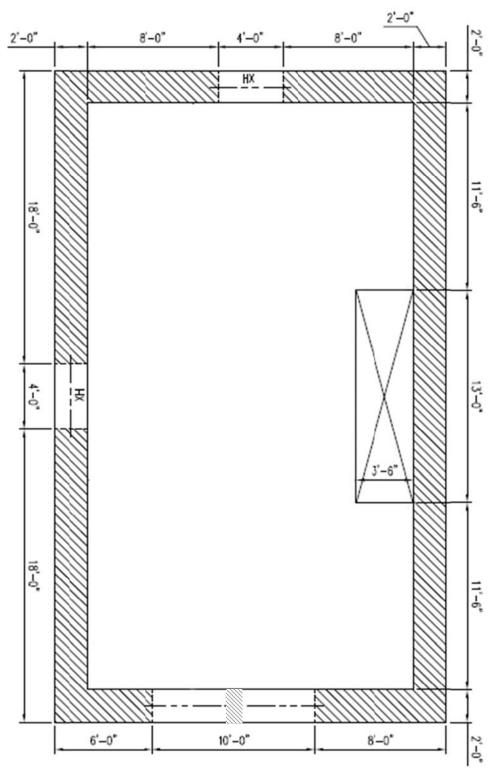
Figure 30. Structure Floor Plan, Basement Level
