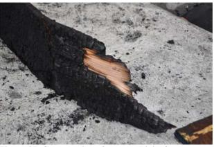
Figure 97 Cross section of ruptured joist from rear section joist adjacent to the stairway.
