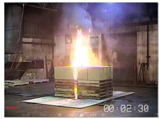
Figure 23. Conditions at 2:30 (150 s) – 400 kW
