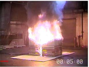
Figure 24. Conditions at 5:00 (300 s) – 2000 kW
