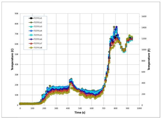
Figure 130. Experiment 4 - First Floor Corner Temperatures
