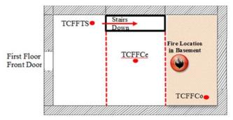
Figure 417. First floor temperature locations and collapse zone
