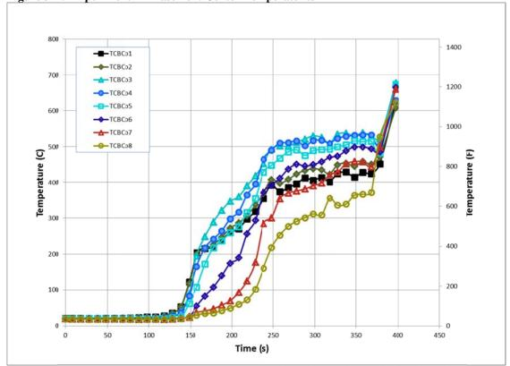
Figure 313. Experiment A - Basement Corner Temperatures
