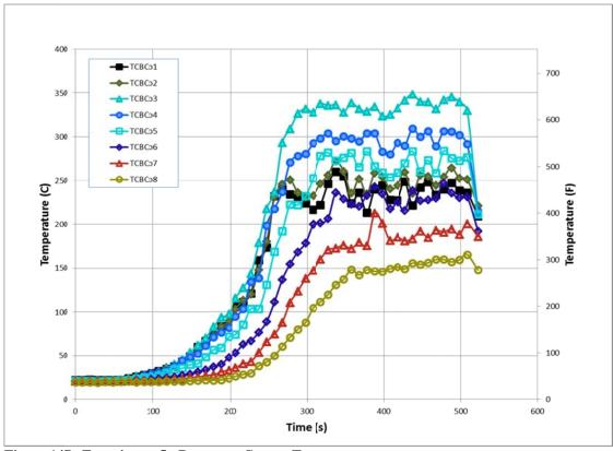
Figure 147. Experiment 5 - Basement Corner Temperatures
