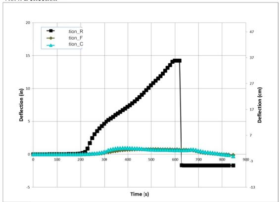
Figure 224. Experiment 8 - Floor System Deflections
