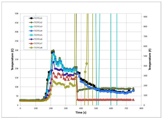
Figure 239. Experiment 9 - First Floor Corner Temperatures
