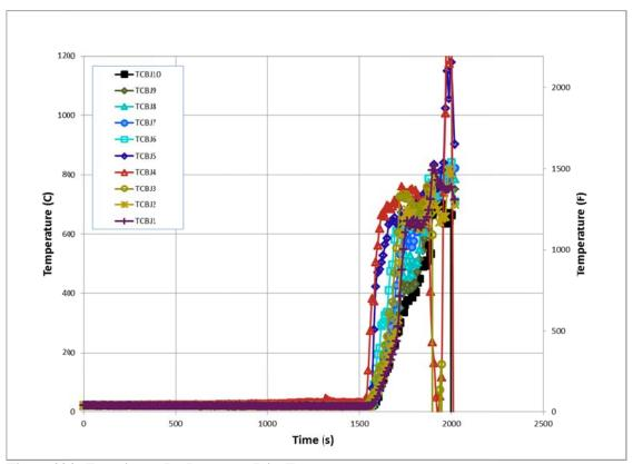
Figure 334. Experiment B - Basement Joist Temperatures
