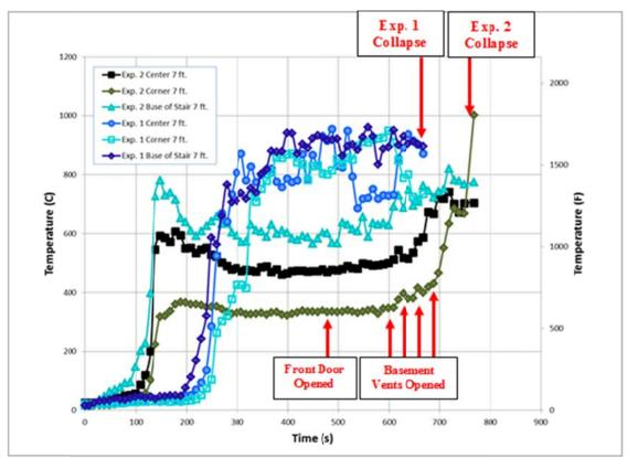
Figure 394. Experiment 1 and 2 Comparison of Basement Temperatures at 7 ft. above the floor
