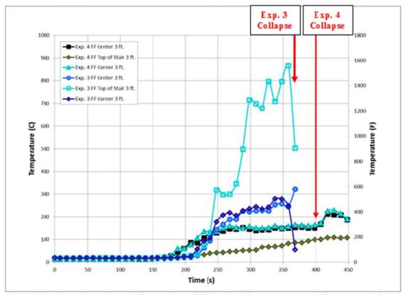
Figure 401. Experiment 3 and 4 Comparison of First Floor Temperatures at 3 ft. above the floor
