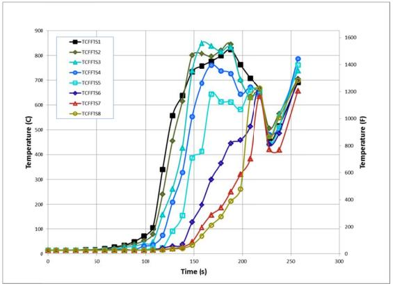
Figure 262. Experiment 10 - First Floor Top of Stair Temperatures
