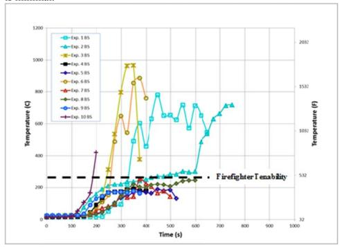
Figure 413 shows the temperatures at the bottom of the stairs up through the time of floor system collapse. It also demonstrates that if the fire is ventilated then the temperatures at the bottom of the stairs are also not tenable for firefighters. The thought that if it is hot at the top of the stairs
