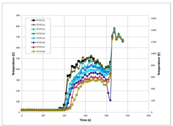
Figure 172. Experiment 6 - First Floor Center Temperatures
