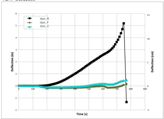
Figure 93. Experiment 2 - Floor System Deflections
