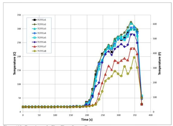
Figure 108. Experiment 3 - First Floor Corner Temperatures
