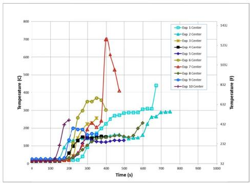
Figure 418. First floor center temperatures 3 ft. above the floor
