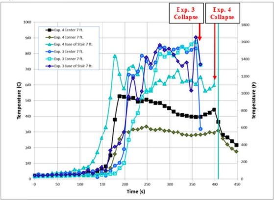
Figure 398. Experiment 3 and 4 Comparison of Basement Temperatures at 7 ft. above the floor
