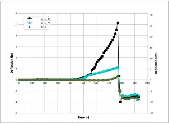
Figure 385. Experiment D - Floor System Deflections
