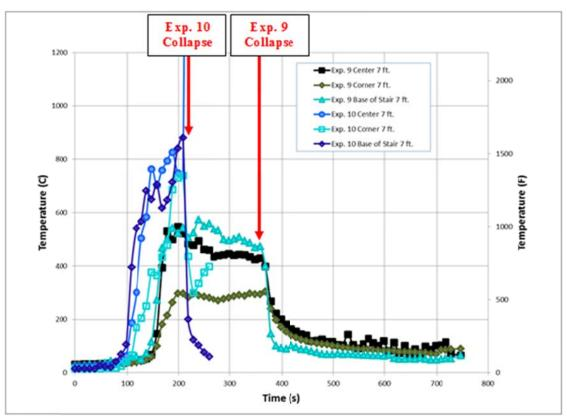
Figure 406. Experiment 9 and 10 Comparison of Basement Temperatures at 7 ft. above the floor
