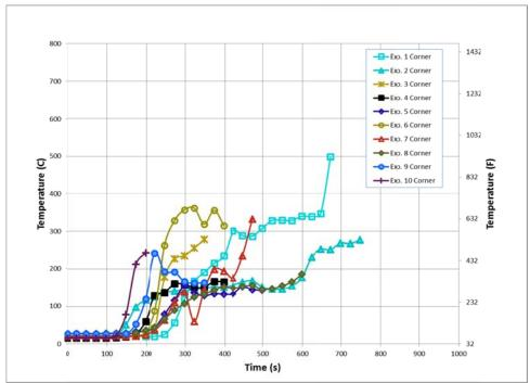
Figure 419. First floor corner temperatures 3 ft. above the floor
