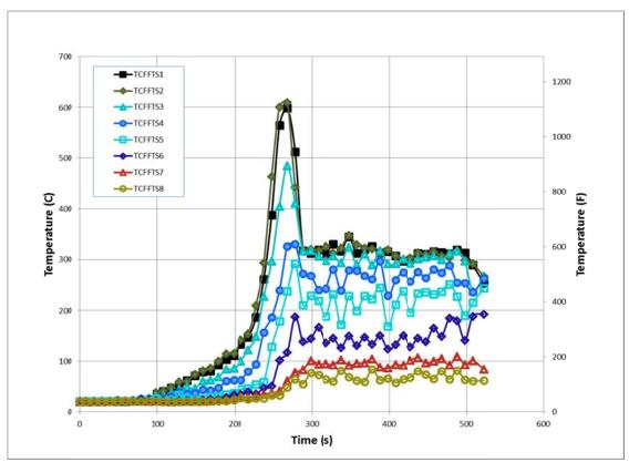
Figure 151. Experiment 5 - First Floor Top of Stair Temperatures
