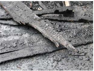
Figure 74 Cross section of ruptured joist from rear section of floor system.
