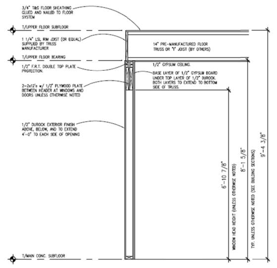
Figure 278. Wall section of experimental structure
