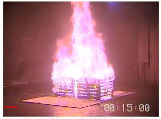
Figure 27. Conditions at 15:00 (900 s) – 4700 kW
