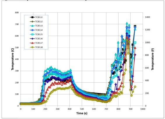
Figure 127. Experiment 4 - Basement Corner Temperatures
