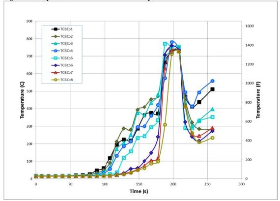
Figure 258. Experiment 10 - Basement Corner Temperatures
