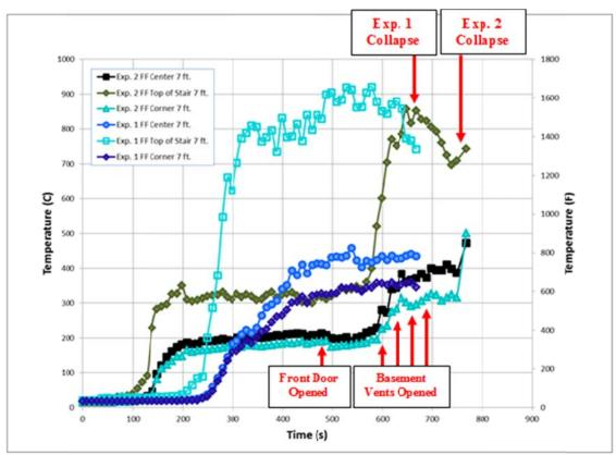
Figure 395. Experiment 1 and 2 Comparison of First Floor Temperatures at 7 ft. above the floor
