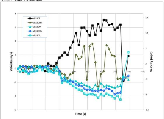
Figure 315. Experiment A - Basement Door Velocities
