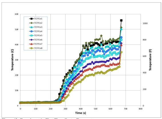
Figure 62. Experiment 1 - First Floor Center Temperatures
