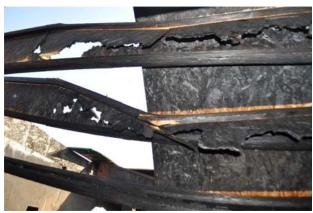
Figure 162 Engineered I-joists web burn-out and flange rupture.
