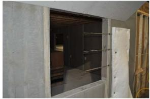
Figure 295. Velocity probe locations in window
