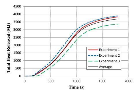
Figure 22. Pallet/Box Total Heat Released
