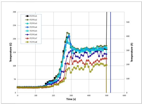
Figure 150. Experiment 5 - First Floor Corner Temperatures
