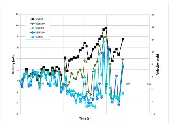
Figure 175. Experiment 6 - Basement Door Velocities
