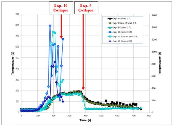
Figure 408. Experiment 9 and 10 Comparison of Basement Temperatures at 3 ft. above the floor Copyright © 2011 Underwriters Laboratories Inc.
