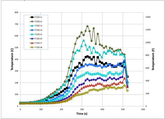
Figure 146. Experiment 5 - Basement Center Temperatures
