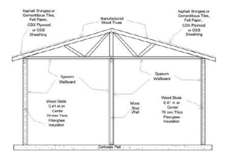
Figure 9. Diagram showing typical construction of the structure.
