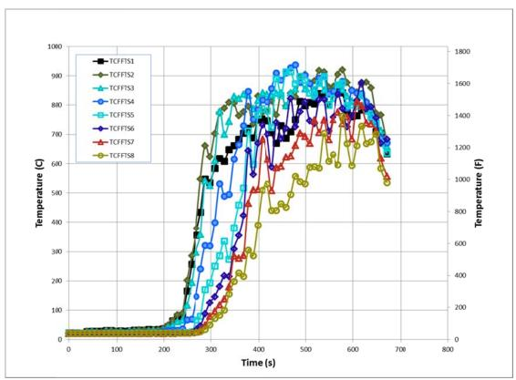
Figure 64. Experiment 1 - First Floor Top of Stair Temperatures
