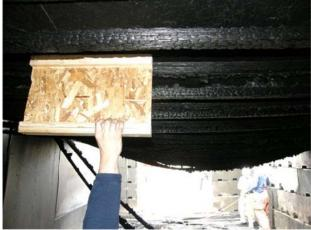
Figure 183 Comparison of original engineered I-joist joist depth to post experiment engineered I-joist depth at front section of floor system.
