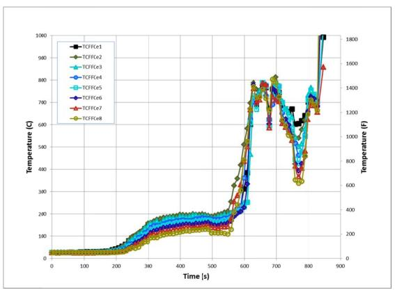
Figure 216. Experiment 8 - First Floor Center Temperatures
