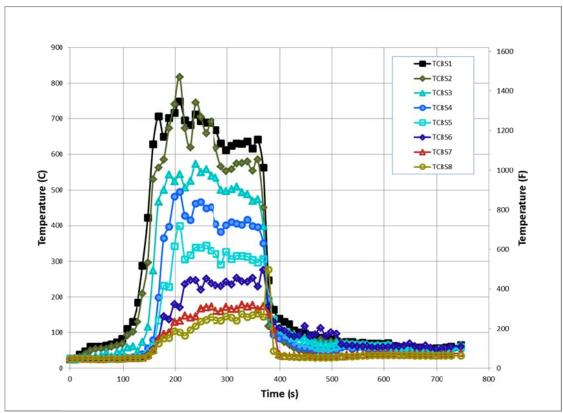
Figure 237. Experiment 9 - Basement Base of Stair Temperatures
