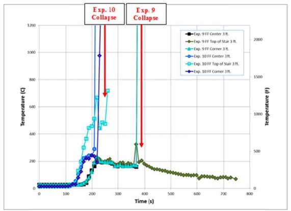
Figure 409. Experiment 9 and 10 Comparison of First Floor Temperatures at 3 ft. above the floor
