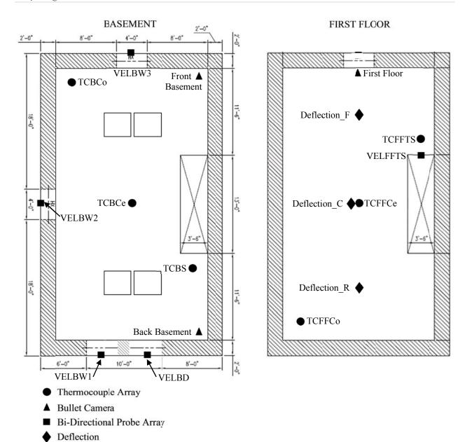
Figure 41. Measurement Locations and Labels
