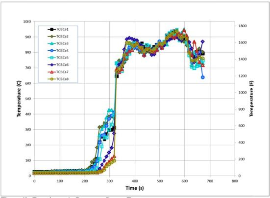
Figure 60. Experiment 1 - Basement Corner Temperatures
