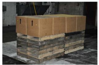
Figure 15. Double stack of fuel load
