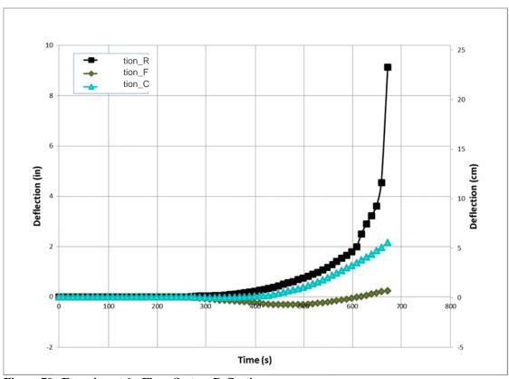
Figure 70. Experiment 1 - Floor System Deflections
