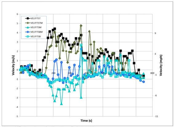
Figure 245. Experiment 9 - First Floor Stair Velocities
