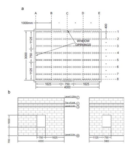
Figure 10. Experimental Compartment: (a) plan; (b) elevation (units in millimeters).
