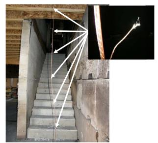
Figure 42. Thermocouple array with detail
