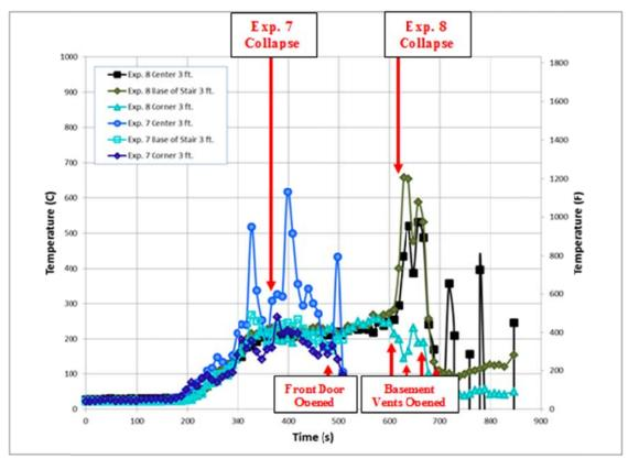
Figure 404. Experiment 7 and 8 Comparison of Basement Temperatures at 3 ft. above the floor
