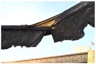
Figure 163 Top chord rupture and internal hinge development at web member butt joint locations.
