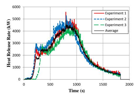
Figure 21. Pallet/Box Heat Release Rates
