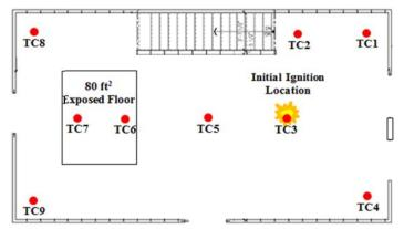
Figure 433. Experiment D Void Thermocouple and Exposed Floor Location
