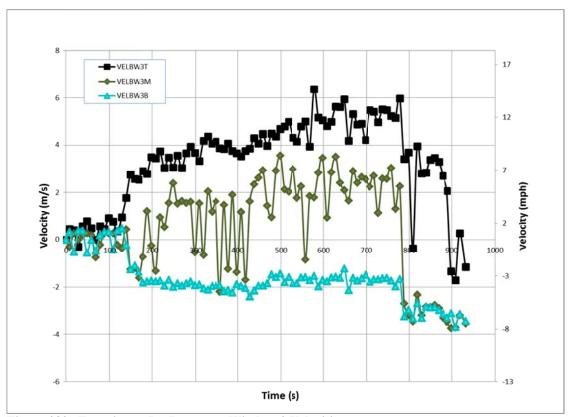
Figure 383. Experiment D - Basement Window 3 Velocities
