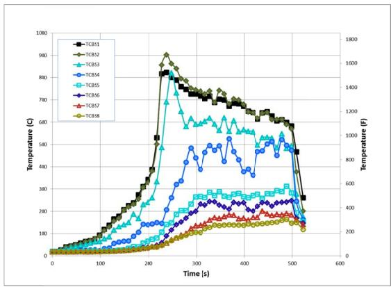
Figure 148. Experiment 5 - Basement Base of Stair Temperatures
