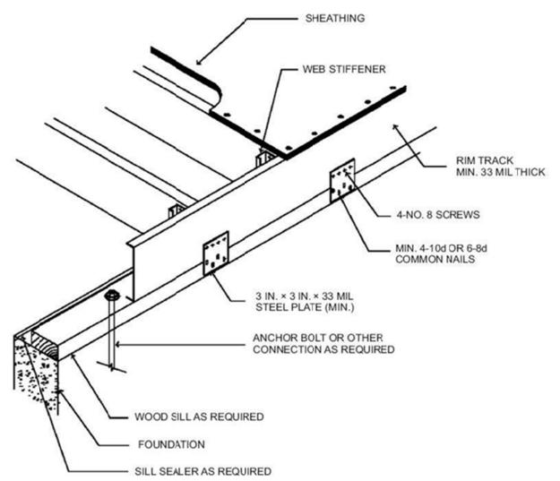
Figure 438. Steel C Joist Detail
