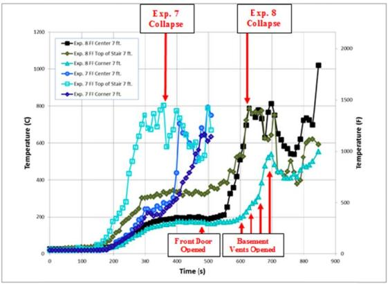
Figure 403. Experiment 7 and 8 Comparison of First Floor Temperatures at 7 ft. above the floor
