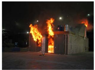
Figure 305. Fire from the ventilation openings
