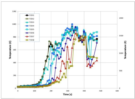
Figure 171. Experiment 6 - Basement Base of Stair Temperatures
