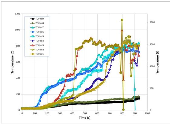
Figure 379. Experiment D - Basement Void Space Temperatures
