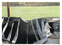
Figure 428. Steel C-joist deformation detail
