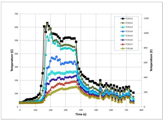
Figure 235. Experiment 9 - Basement Center Temperatures
