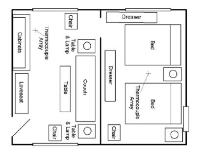
Figure 8. Plan view of generic test structure showing approximate placement of furniture and other items with the structure (not to scale).
