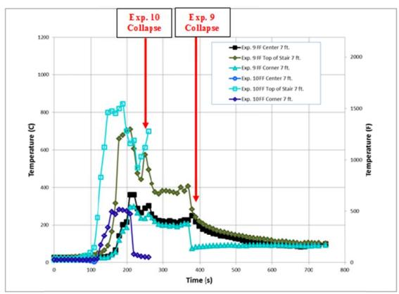
Figure 407. Experiment 9 and 10 Comparison of First Floor Temperatures at 7 ft. above the floor
