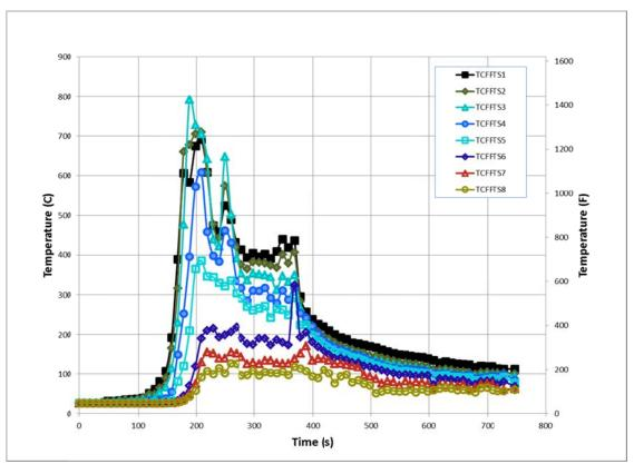
Figure 240. Experiment 9 - First Floor Top of Stair Temperatures
