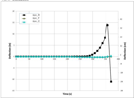
Figure 115. Experiment 3 - Floor System Deflections
