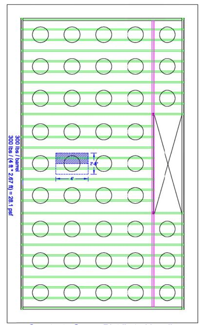
Constant - Span - Distributed Loading 2x12 Solid-Sawn = #2 HF KD @ 16" o.c.
