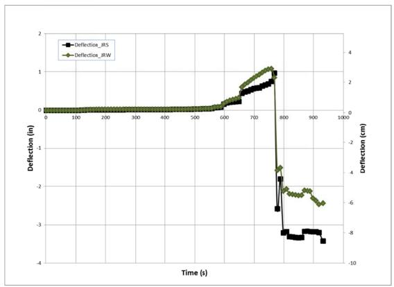
Figure 386. Experiment D - Floor System Deflections
