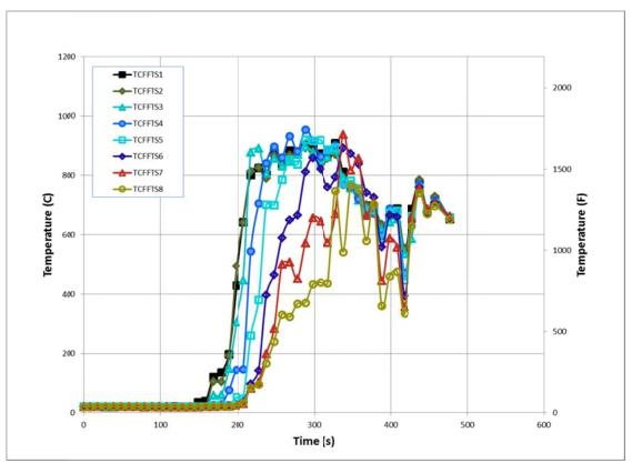
Figure 174. Experiment 6 - First Floor Top of Stair Temperatures
