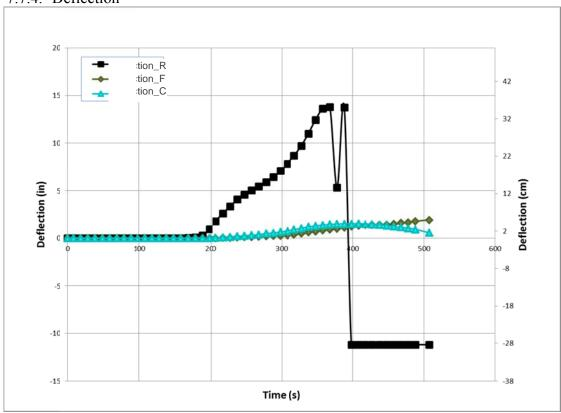
Figure 202. Experiment 7 - Floor System Deflections
