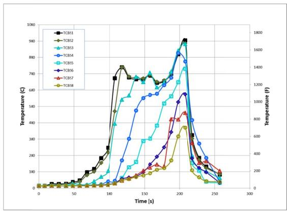
Figure 259. Experiment 10 - Basement Base of Stair Temperatures
