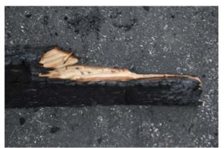
Figure 96 Cross section of ruptured joist from rear section joist.
