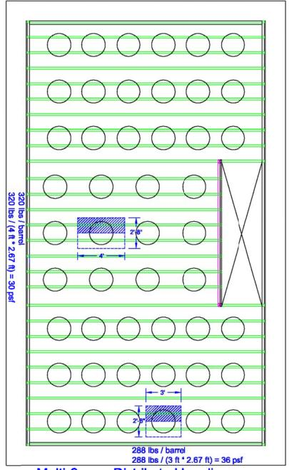
Multi-Span - Distributed Loading I-Joist = 11-7/8 BCI 60s - 2.0 @ 16" o.c.
