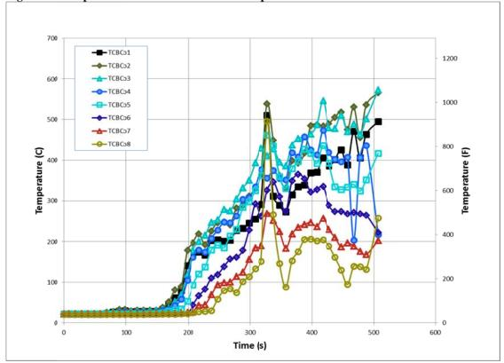
Figure 192. Experiment 7 - Basement Corner Temperatures
