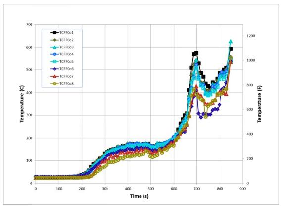
Figure 217. Experiment 8 - First Floor Corner Temperatures
