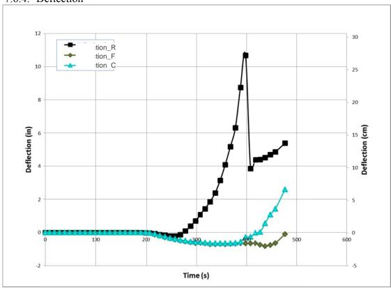
Figure 180. Experiment 6 - Floor System Deflections
