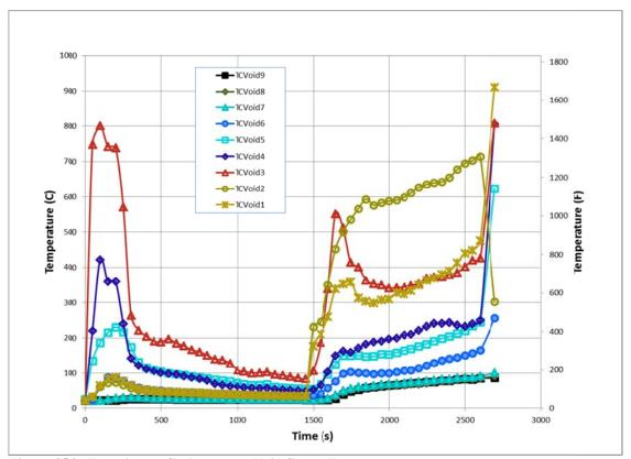
Figure 354. Experiment C - Basement Void Space Temperatures
