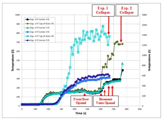
Figure 397. Experiment 1 and 2 Comparison of First Floor Temperatures at 3 ft. above the floor
