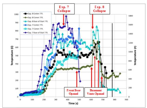
Figure 402. Experiment 7 and 8 Comparison of Basement Temperatures at 7 ft. above the floor
