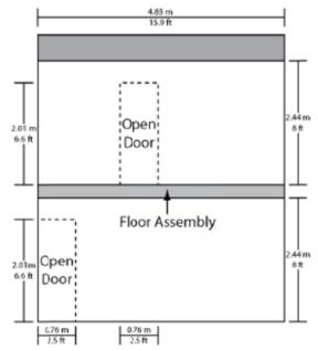
Figure 12. Elevation view of the structure, looking North, with dimensions.
