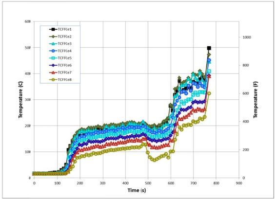
Figure 85. Experiment 2 – First Floor Center Temperatures
