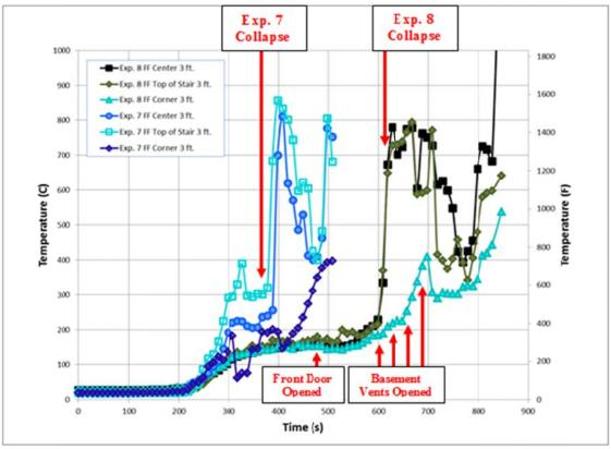
Figure 405. Experiment 7 and 8 Comparison of First Floor Temperatures at 3 ft. above the floor
