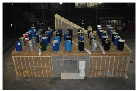
Figure 304. Barrel loading placement
