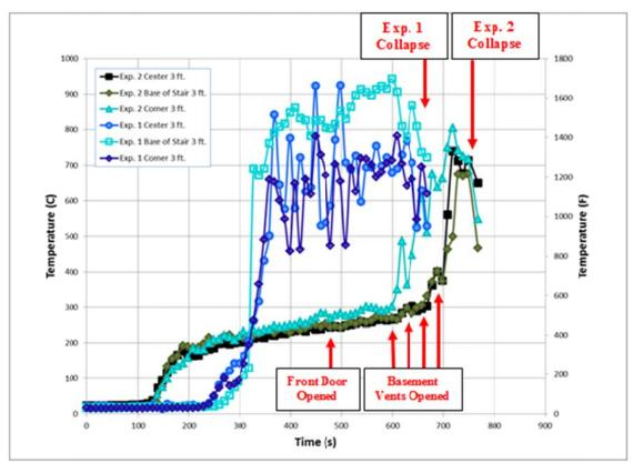
Figure 396. Experiment 1 and 2 Comparison of Basement Temperatures at 3 ft. above the floor
