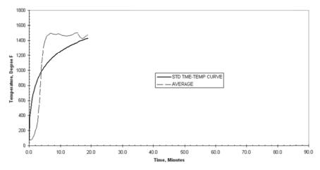
Figure 7 - UL263 Standard Time Temperature Curve and Average Furnace Temperature vs. Time for Assembly No. 1
