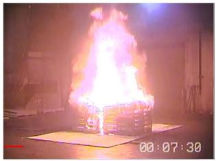
Figure 25. Conditions at 7:30 (450 s) - 2400 kW
