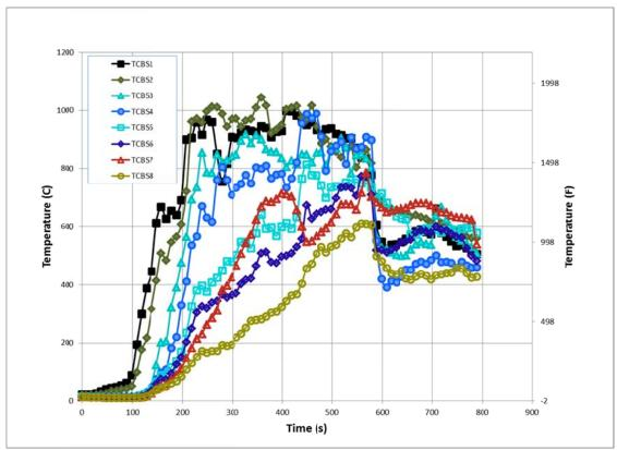
Figure 378. Experiment D - Basement Base of Stair Temperatures
