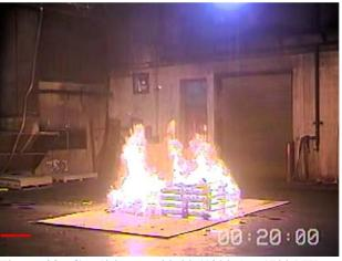
Figure 28. Conditions at 20:00 (1200 s) – 1700 kW
