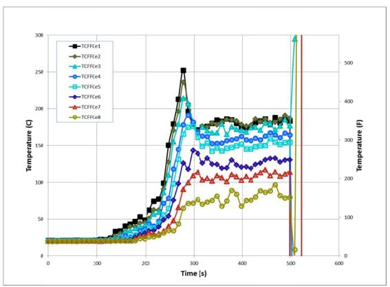
Figure 149. Experiment 5 - First Floor Center Temperatures
