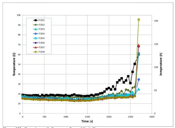
Figure 353. Experiment C- Basement Base of Stair Temperatures
