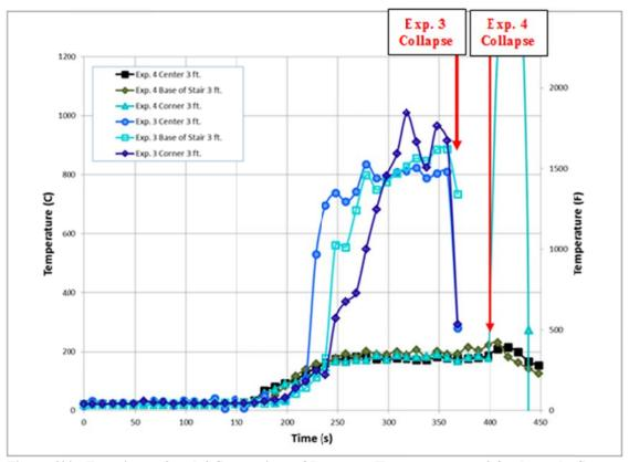
Figure 400. Experiment 3 and 4 Comparison of Basement Temperatures at 3 ft. above the floor
