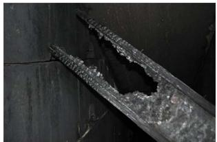
Figure 117 The web burn-out induced causing complete rupture of the chord members at center span.
