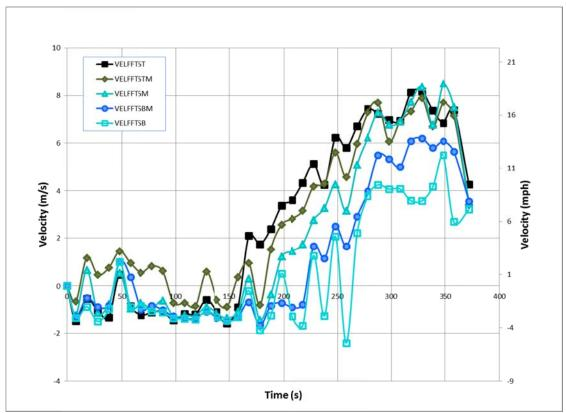
Figure 114. Experiment 3 - First Floor Stair Velocities
