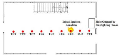
Figure 429. Experiment C Void Thermocouple and Hole Location
