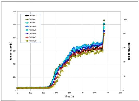
Figure 63. Experiment 1 - First Floor Corner Temperatures
