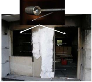
Figure 43. Velocity probe locations in doorway and window with detail
