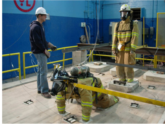
Figure 19 Picture from floor test showing mechanical loading conditions
