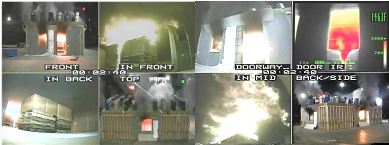
Figure 20 Video and IR camera records of basement fire test at 2:40 minutes
