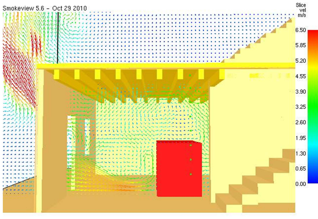
Figure 38 Velocity contours at a plane intersecting the middle of the basement door
