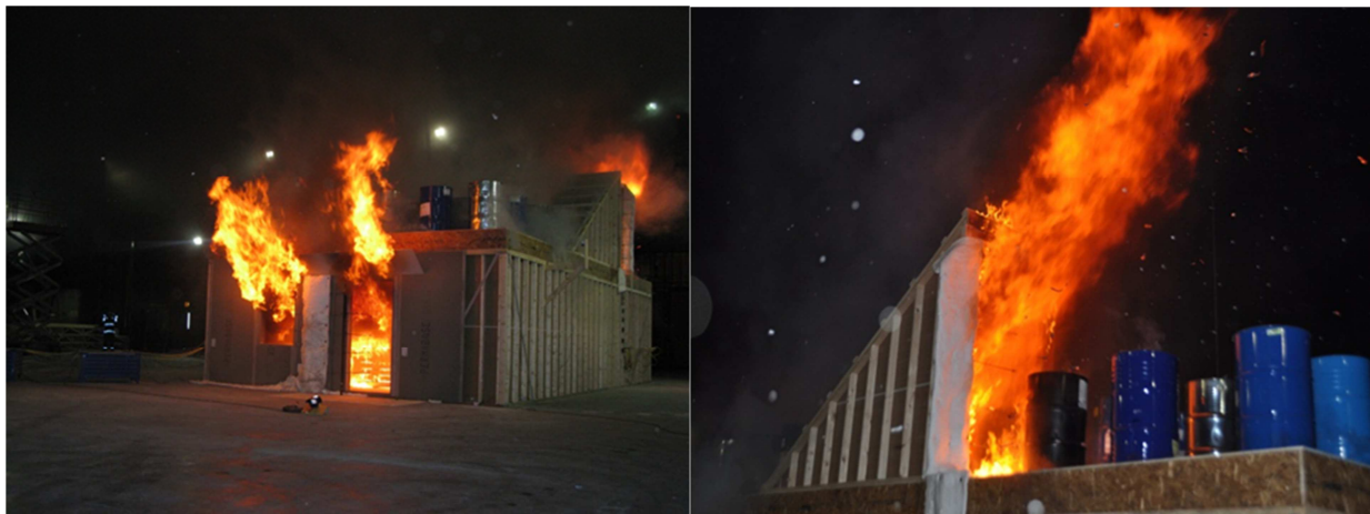
Figure 15 Pictures of flames through openings: front (left) stairway door at top (right)
