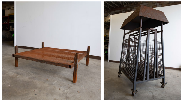
Figure 1. Training fuel racks used for heat release rate characterization experiments. Left image is the rack used for 20 of the 21 training fuel packages. Right image is the modified rack used for the remaining fuel package.
