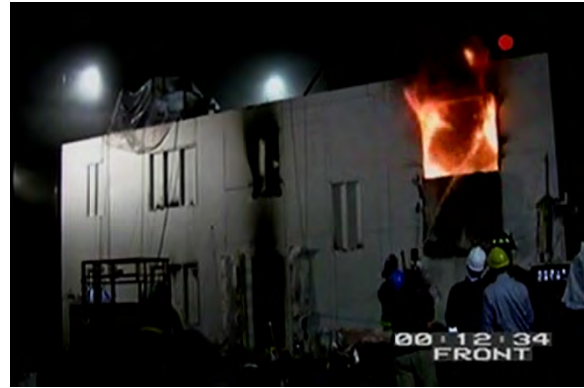
Figure 6.28: Water being applied from outside the house
