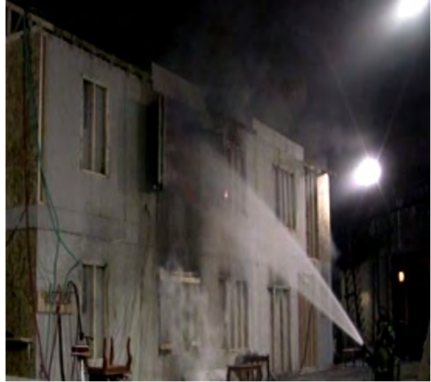
Figure 6.36: Fog Stream Sealing Flow Path
