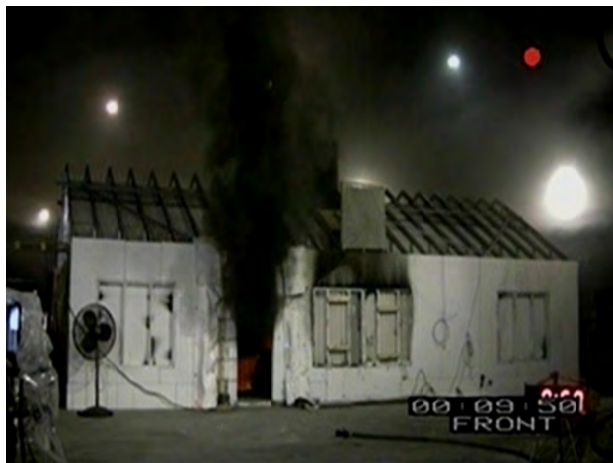
Figure 6.5: 5 seconds after roof vent
