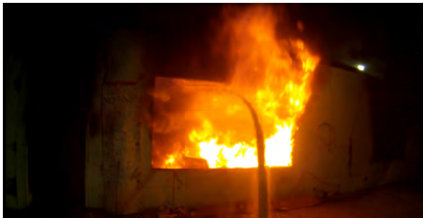
Figure 5.539: Start of Straight Stream Application
