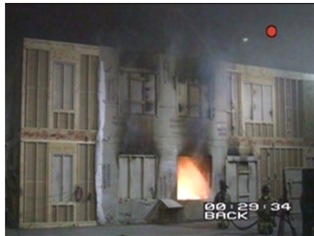
Figure 5.546: Fog Stream Application
