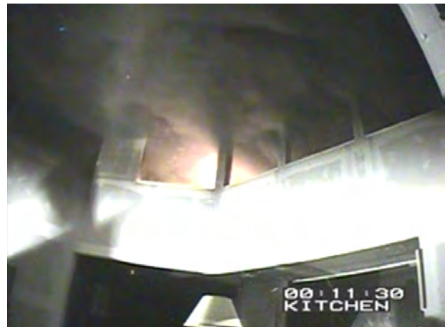
Figure 5.478: Exp. 14 thirty seconds after roof ventilation looking up to Bedroom fire
