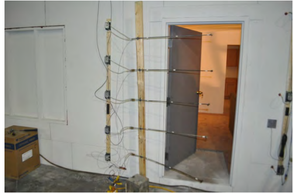
Figure 5.26: Doorway Velocity Probes
