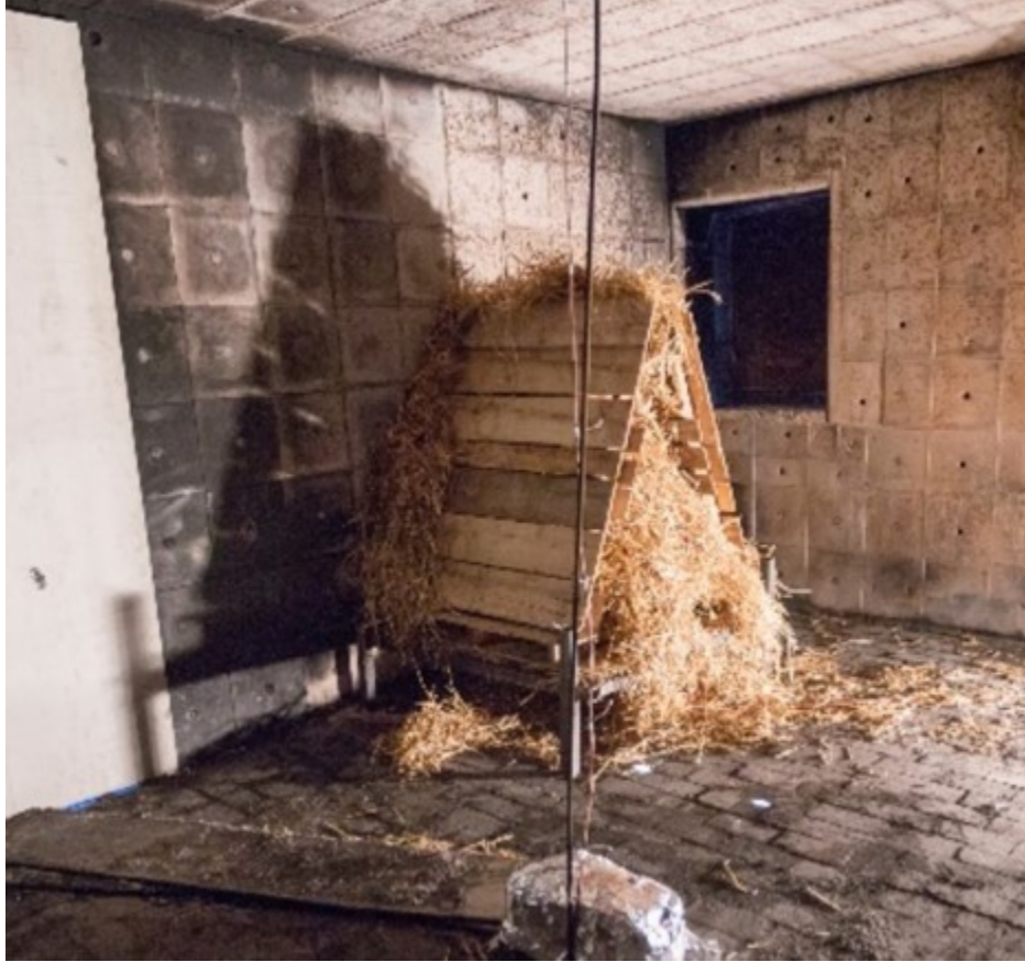
Figure 3.2: Pallets and Straw Fuel Package
