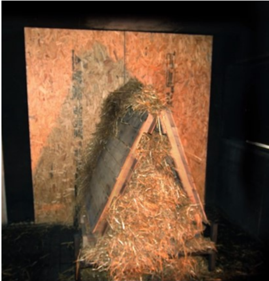
Figure 3.3: Pallets, Straw, and OSB Fuel Package
