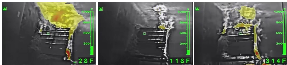
Figure 5.1: Comparison of IR view 60 seconds after ignition in fire room for Pallets Experiments 1 (left), 2 (center), and 3 (right). Note that in Pallets Experiment 2, the burning is concentrated on the side of the fuel package away from the wall, while the burning for the other two experiments is more uniform throughout the fuel package. This explains the slower growth rate observed in Pallets Experiment 2.
