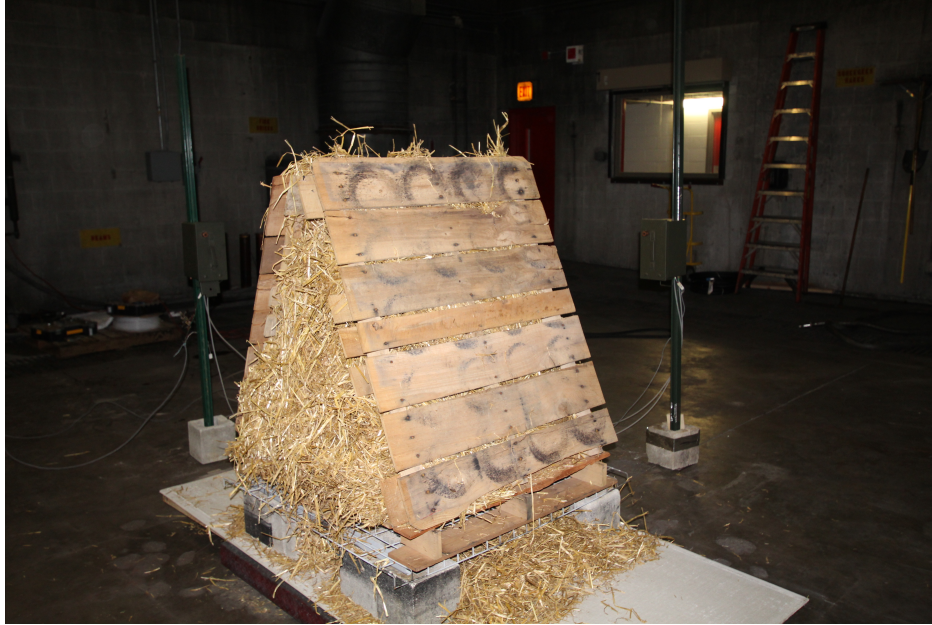
Figure 3.5: Pallets and Straw Free Burn Assembly
